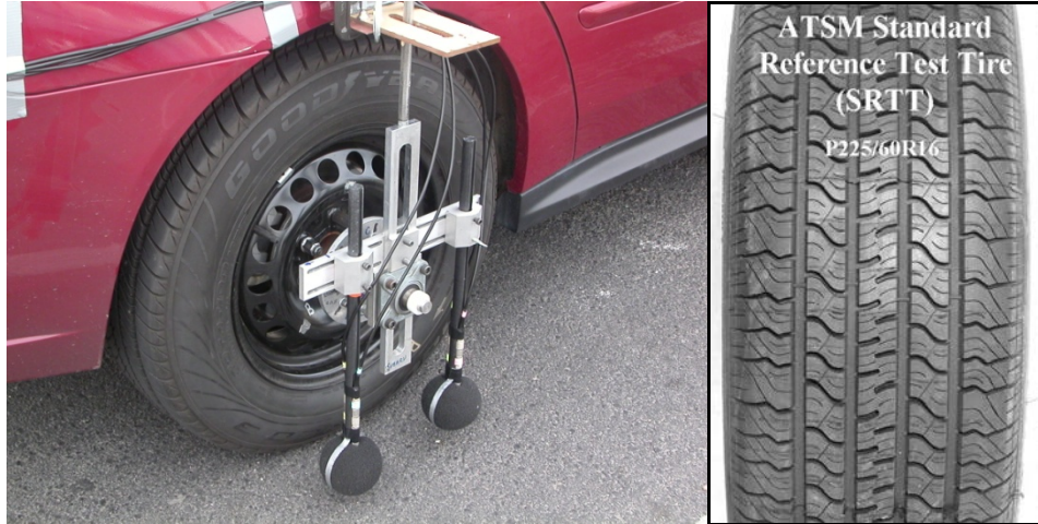
Figure 16. OBSI dual probe system and the SRTT.
