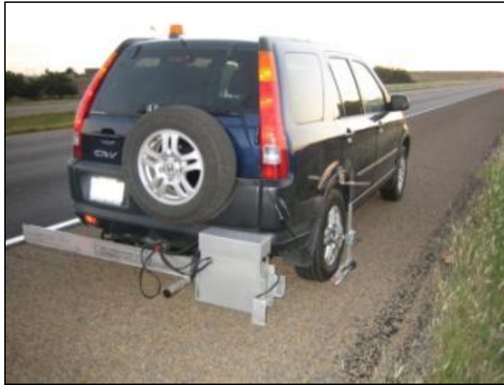
Figure 30. High-speed inertial profiler mounted behind the test vehicle.
