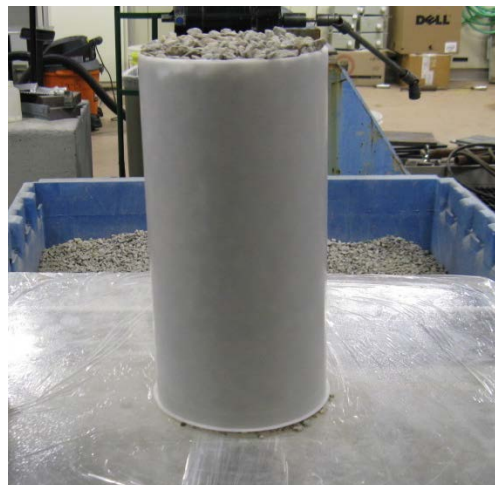
Figure 7. Photo. Repose angle cylinder test.
