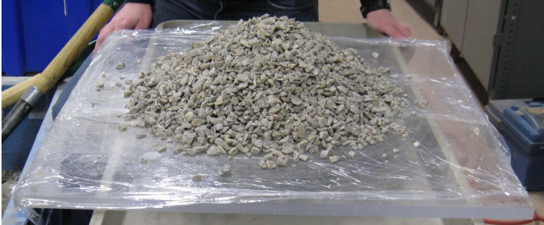
Figure 8. Photo. Aggregate pile to determine repose angle.
