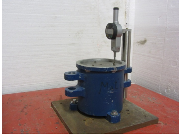
Figure 6. Photo. LVDT and mold set-up for vibratory table tests.
