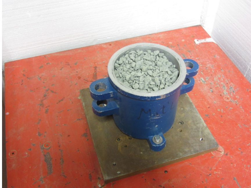
Figure 5. Photo. Mold (0.1 ft 3 ) for funnel and vibratory table tests.
