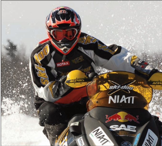
The direct-injected, two-stroke-powered snowmobile uses ethanol fuel, reduces pollution emissions, and decreases sound emissions while maintaining stock power and handling characteristics. (photo: © Michigan Technological University)
