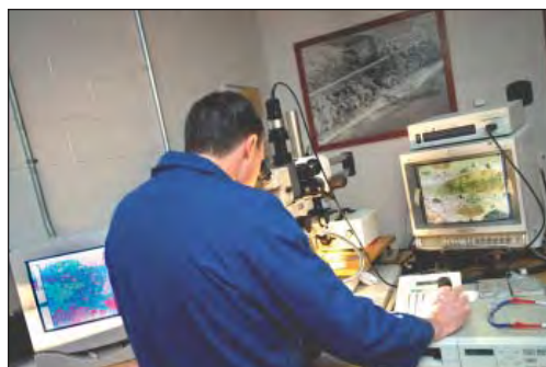
UTC-MiSTI graduate student using a stereo optical microscope to perform the ASTM C457 test on a concrete pavement sample in the Material Characterization Facility at Michigan Technological University.
