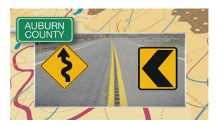
The county received funding and implemented low-cost strategies, such as warning signs, chevron signing, and raised pavement markers. The county even added non-traditional "curve ahead" pavement markings, including directional arrows as a
