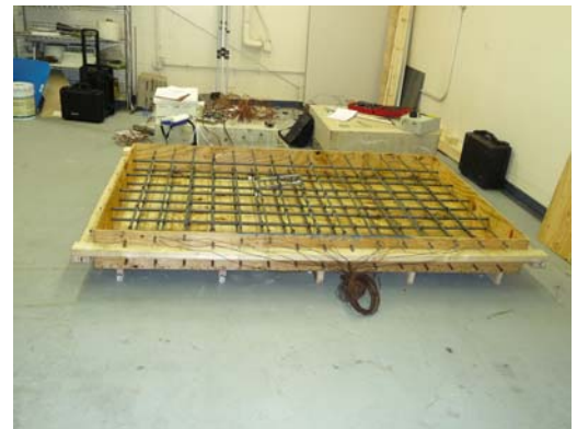
Figure 6. Photo. Bridge deck specimen with reinforcing bars.
