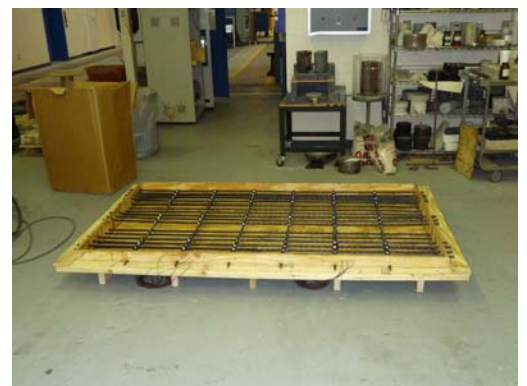
Figure 7. Photo. Prestressed concrete specimen with untensioned tendon strands.
