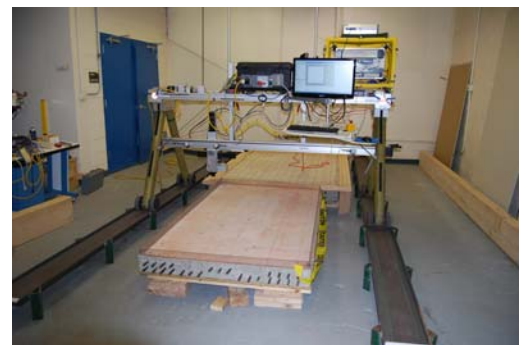
Figure 8. Photo. Half-automated scanner with bridge deck specimen with reinforcing bars (top) and specimen with prestressing tendons (bottom).
