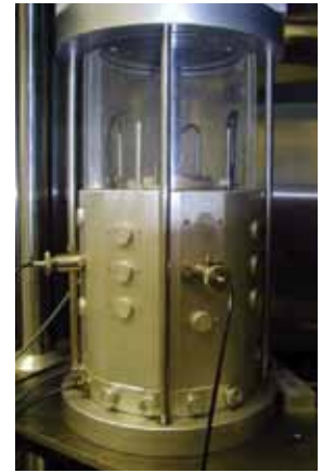
A dynamic modulus testing apparatus (courtesy North Carolina State University).
