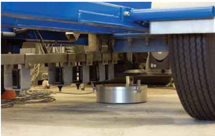
Left: Calibrating an FWD. The reference load cell is positioned under the FWD load plate.
