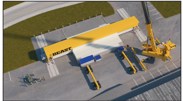
Aerial concept image of the BEAST, the world's first facility to quantitatively measure the effects of environmental and traffic loading on full-scale bridge sections in a greatly compressed time frame. The BEAST will be completed this coming spring.
