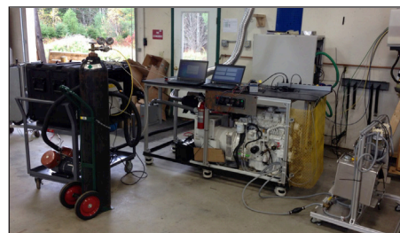
Figure 2. Engine test assets. Top : 41 ft Maine Maritime Academy utility vessel Quickwater equipped with two 360 hp Cummins marine diesel engines. Bottom : Lab-operated Caterpillar C2.2 marine diesel generator.
