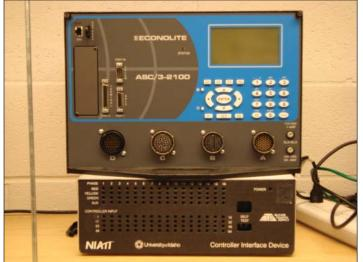
Econolite ASC/3 traffic controller atop NIATT controller interface device (CID)
