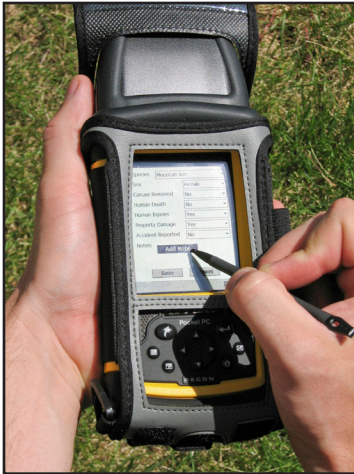
An integrated PDA-GPS handheld data collector developed for the ROCS project.
