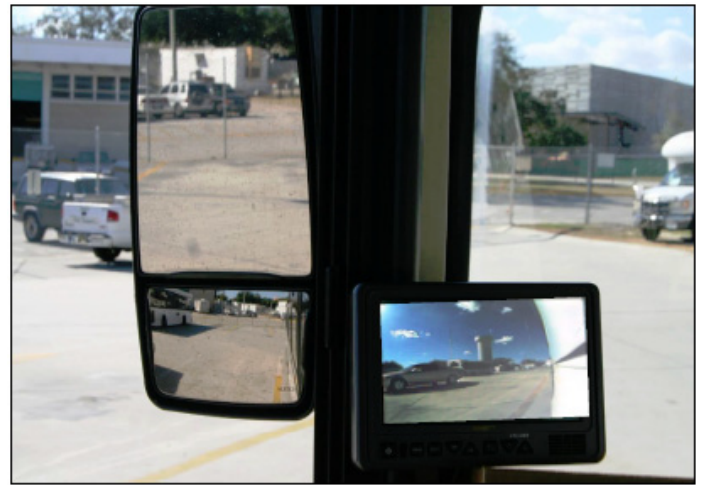
Vehicle visible with video system, but not with mirrors.
