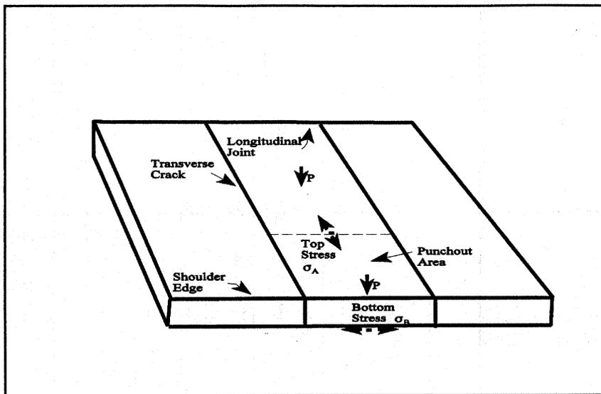
Figure 18. Critical wheel load stresses in a loaded CRC pavement system.<sup>(2)</sup>
