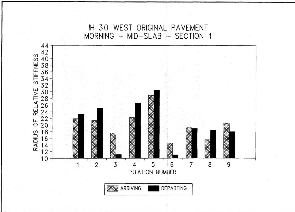
Figure 31. Radius of relative stiffness versus station (I-30W, morning, mid-slab, section 1).
