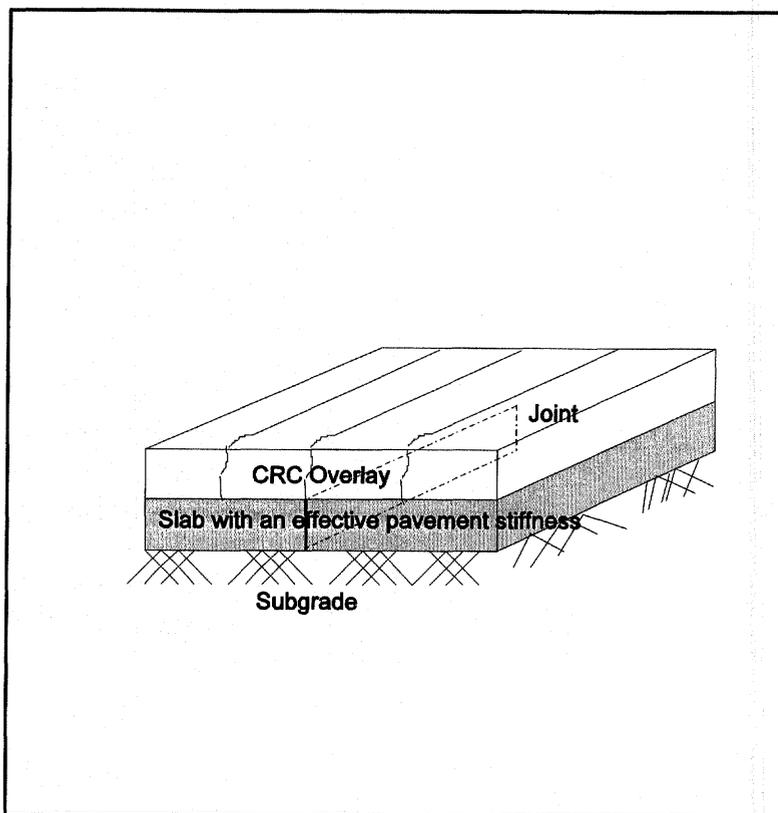
Figure 23. Section of the slab with the overlay.
