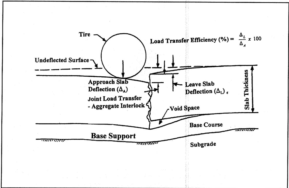
Figure 17. Load transfer efficiency.<sup>(51)</sup>
