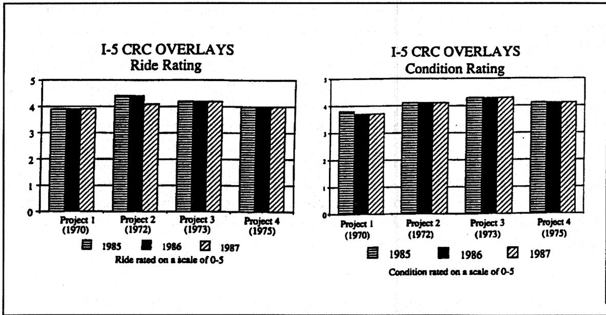
Figure 7. Ride rating and condition rating.<sup>(32)</sup>
