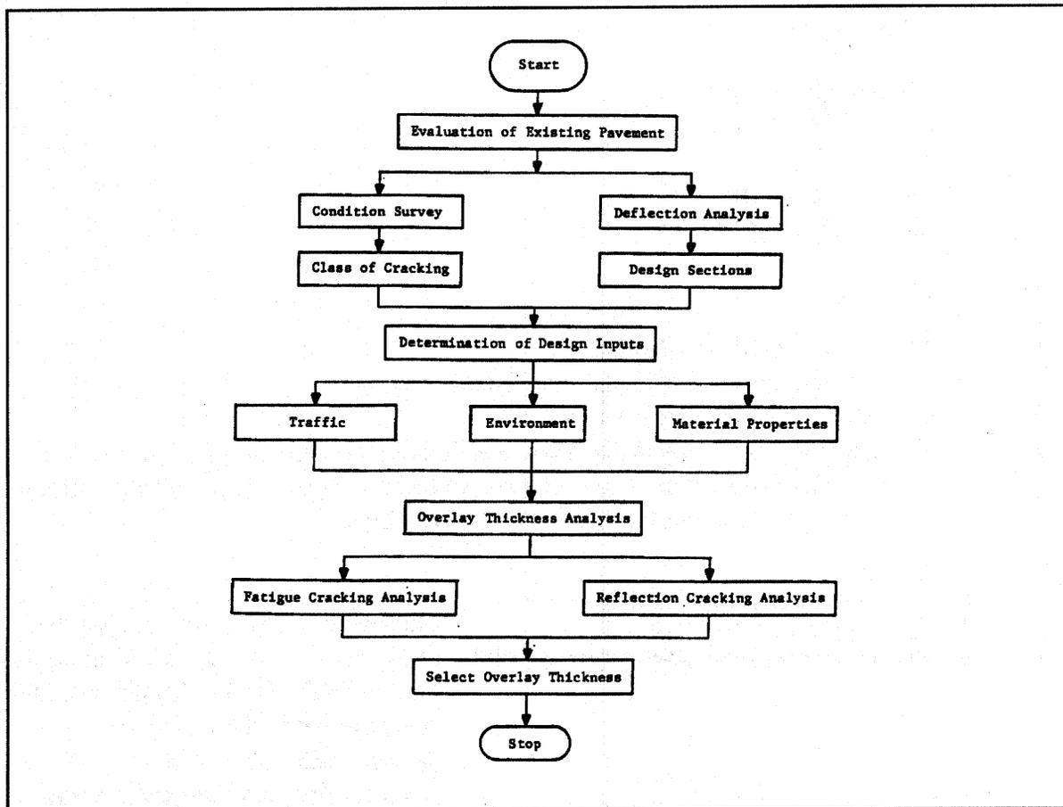
Figure 13. Flow chart of the FHWA/Texas design procedure.<sup>(14)</sup>
