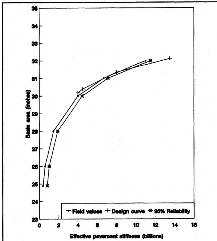
Figure 28. Effective pavement stiffness requirements at 95 percent reliability.
