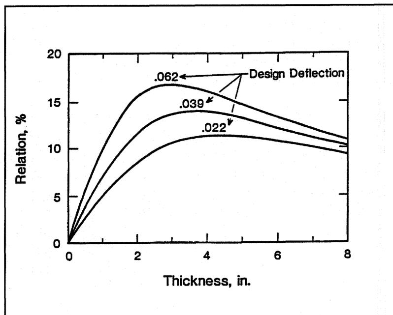
Figure 4. Percent reduction of deflection per inch of thickness.<sup>(17)</sup>
