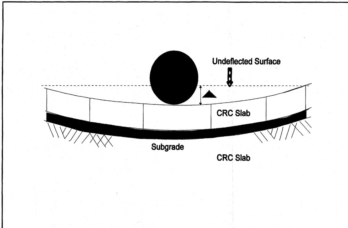
Figure 15. Shape of the deflection basin under a slab of high stiffness and weak subgrade support.
