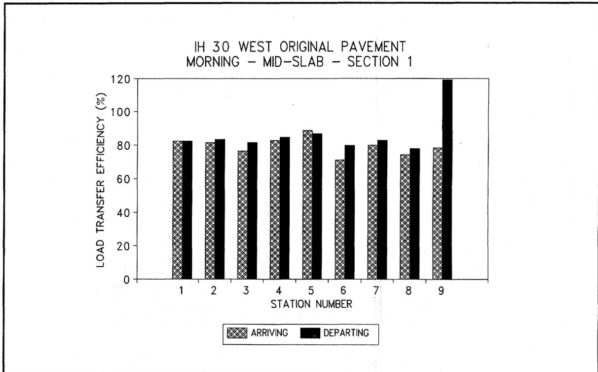
Figure 32. Load transfer efficiency versus station (I-30W, morning, mid-slab, section 1).
