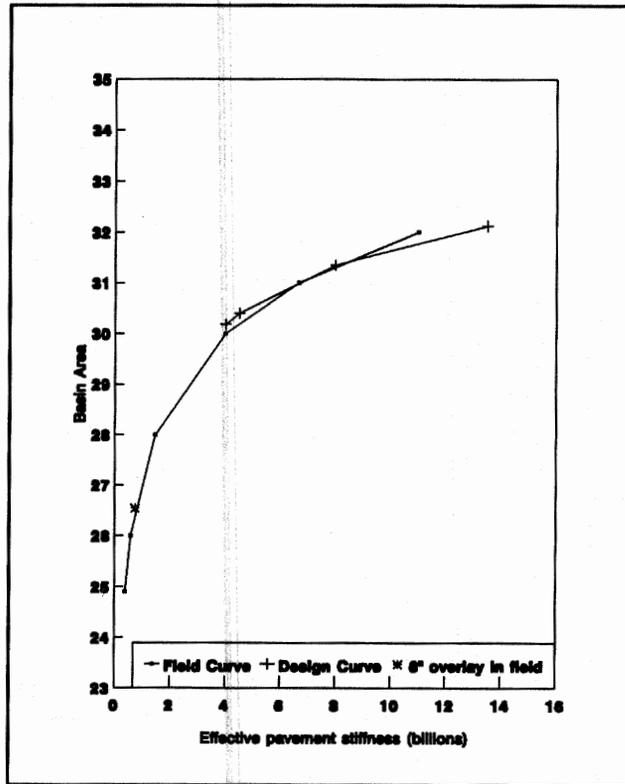
Figure 25. Design criteria based on effective pavement stiffness.
