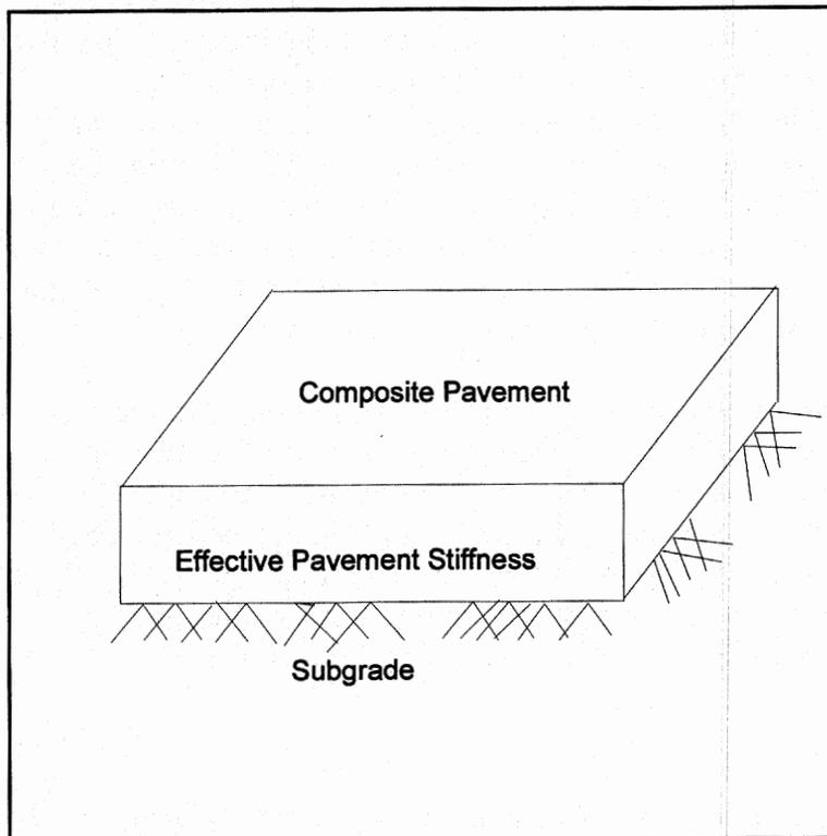
Figure 22. Section of the composite pavement.
