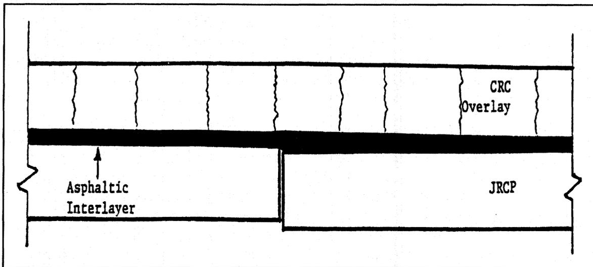
Figure 8. Longitudinal section of overall pavement structure at joint in JRCP illustrating cantilevering of CRC overlay because of differential vertical movement of JRCP slabs opposite joint.<sup>(37)</sup>
