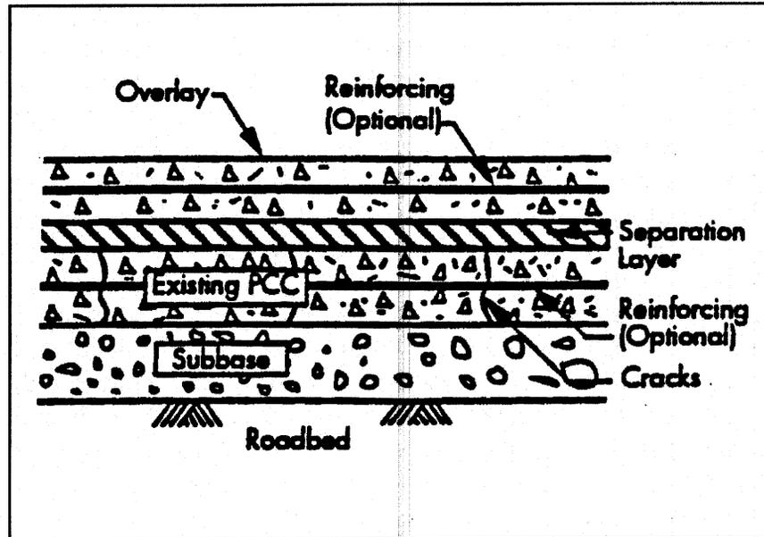
Figure 1. Unbonded concrete overlay.<sup>(11)</sup>
