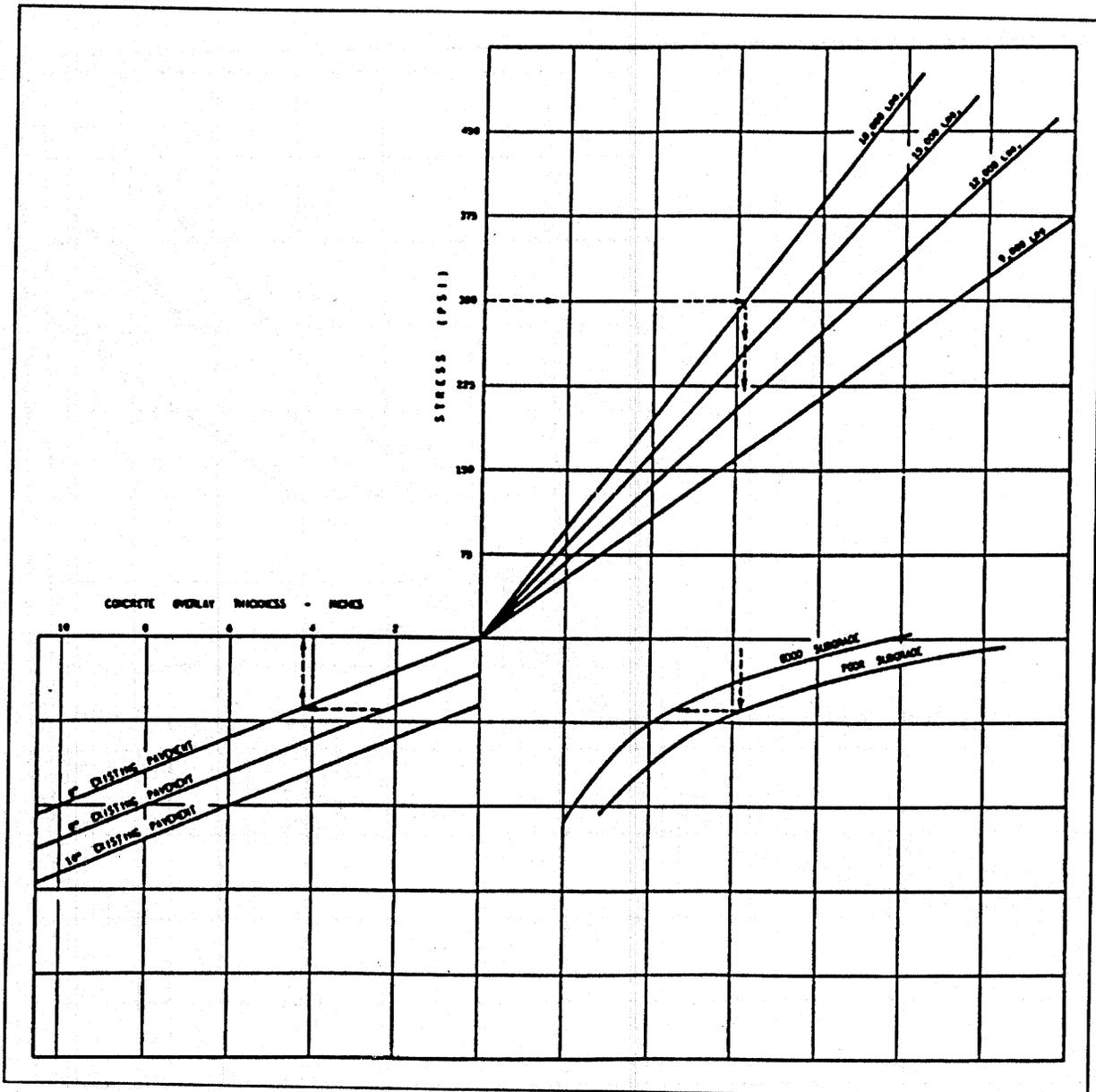
Figure A-2. Design chart for CRC overlay (partially bonded).<sup>(18)</sup>
