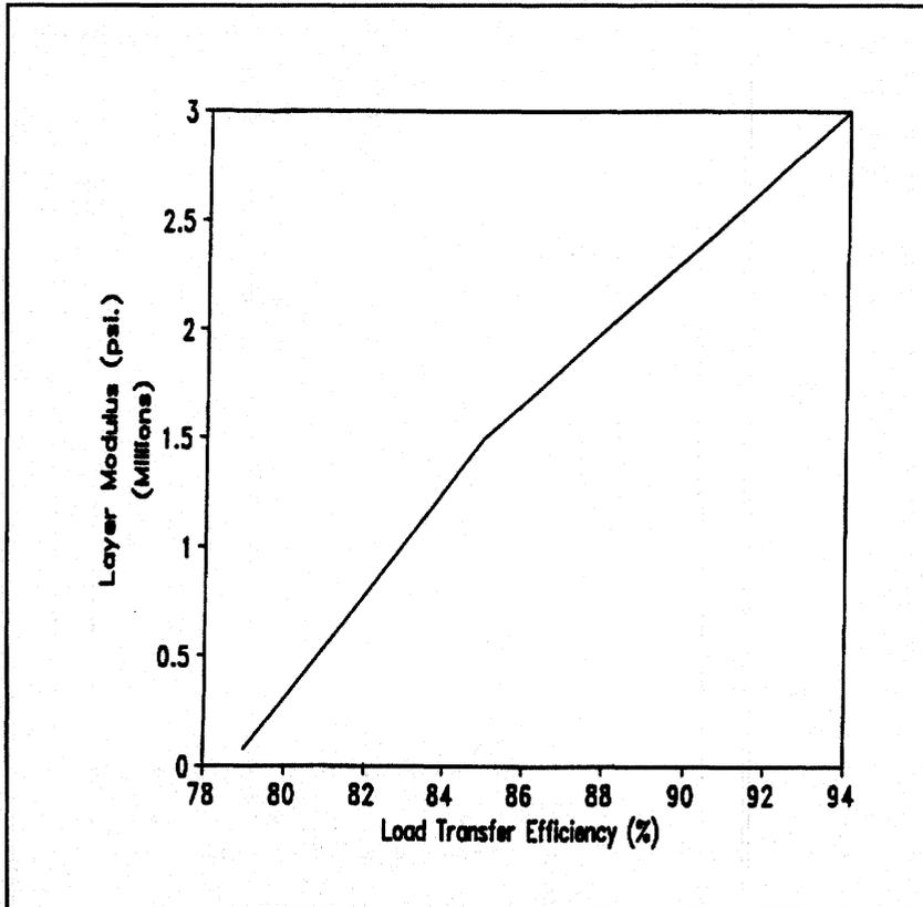
Figure 24. Variation of load transfer with layer modulus.
