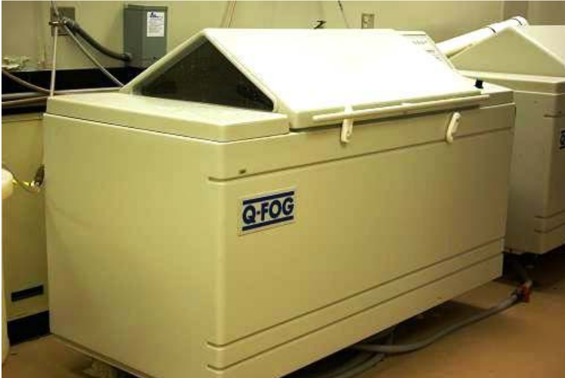
Figure 4. Photo. Salt-fog chamber.
