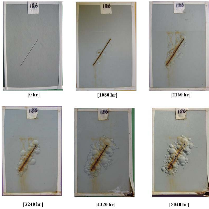
Figure 44. Photo. Progressive changes of panel 186 (WBEP: ALT).
