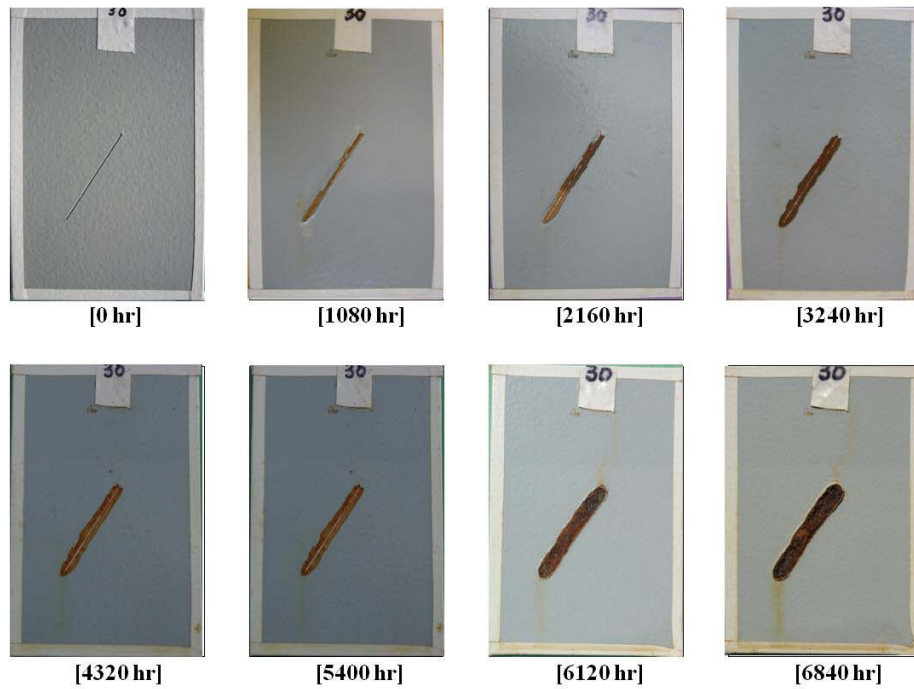
Figure 23. Photo. Progressive changes of panel 30 (two-coat: ALT).
