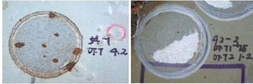
Figure 18. Photo. Cohesive failure modes of ASP and EM.
