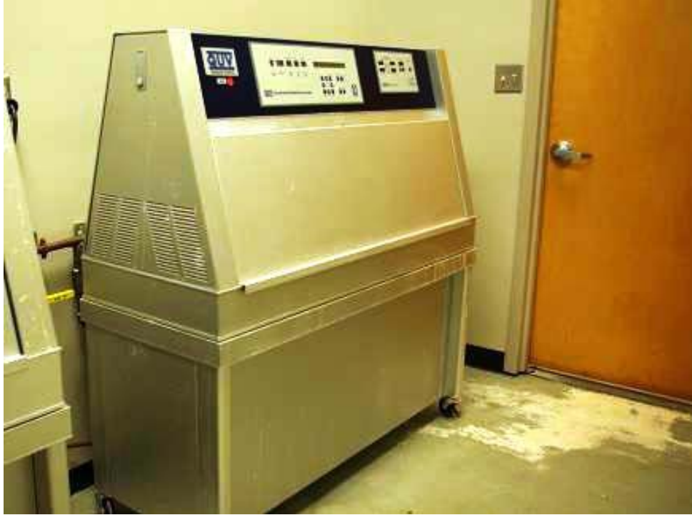
Figure 5. Photo. UV weathering tester.
