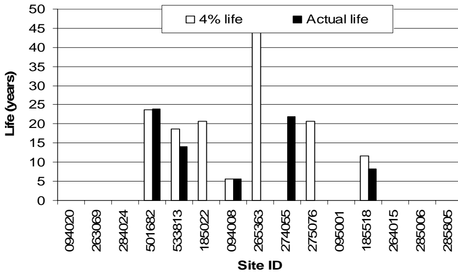
Figure 16. Pavement life prediction comparison between actual annual AADTT growth rate and 4 percent annual AADTT growth rate, rigid pavement sites.
