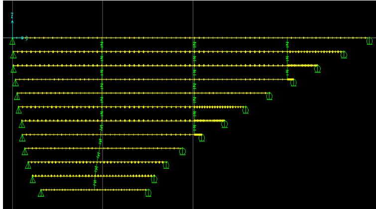
Figure 41. Image. Finite element model for the stay cable system of the Fred Hartman Bridge in Houston, TX.
