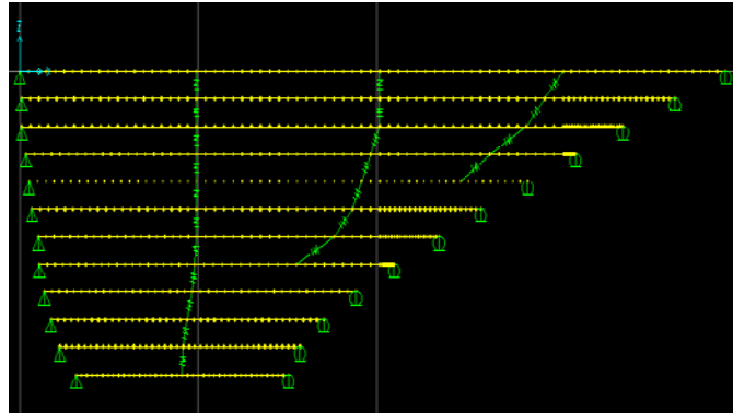
Figure 50. Image. Finite element model for the stay cable system with a varied crosstie configuration (variation 1).
