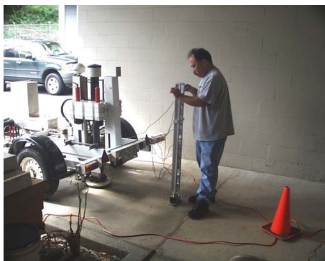
Figure 3. On-Site FWD Calibration in Hawaii
