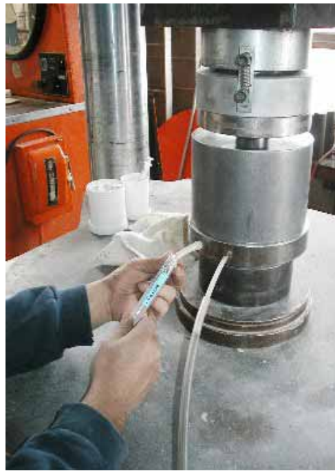
Figure 17. Pore fluid being collected from die set.
