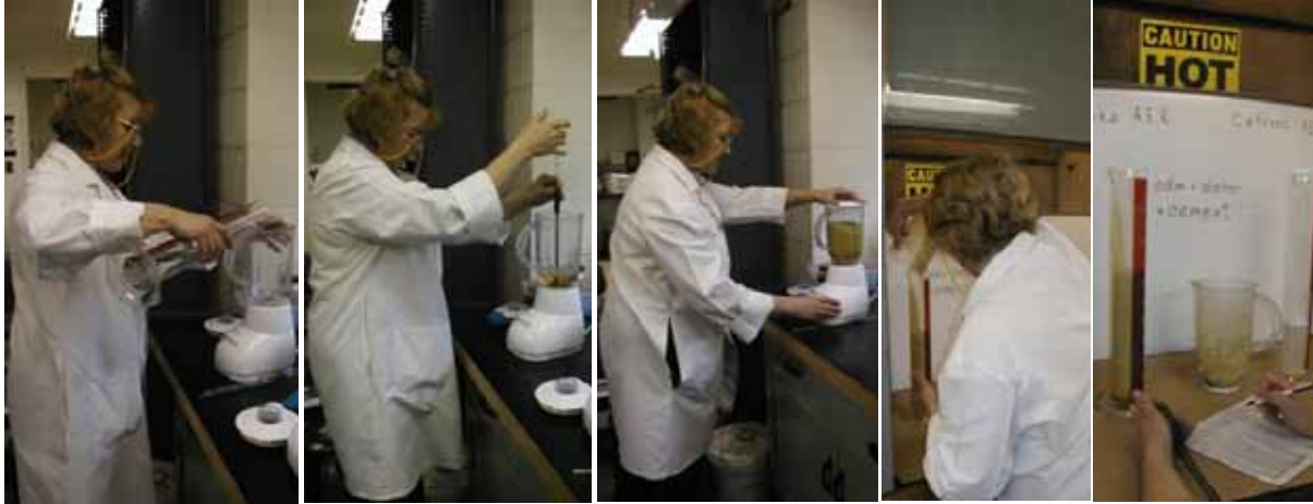
Figure 41. Foam drainage procedure.
