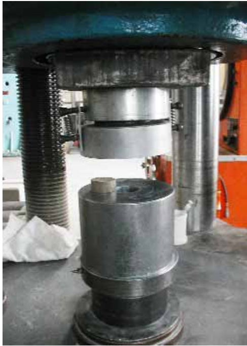
Figure 16. Die set for squeezing pore solution from hardened cement paste specimens.
