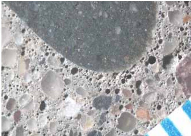
Figure 47. Rating 3, severe clustering. Visual rating guide for analysis of air void clustering severity (PCA R&D Serial No. 2789).
