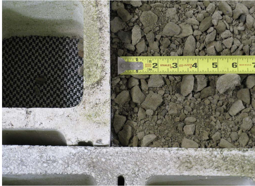
Figure 5. Photo. Sample of VDOT 21-A gravel.
