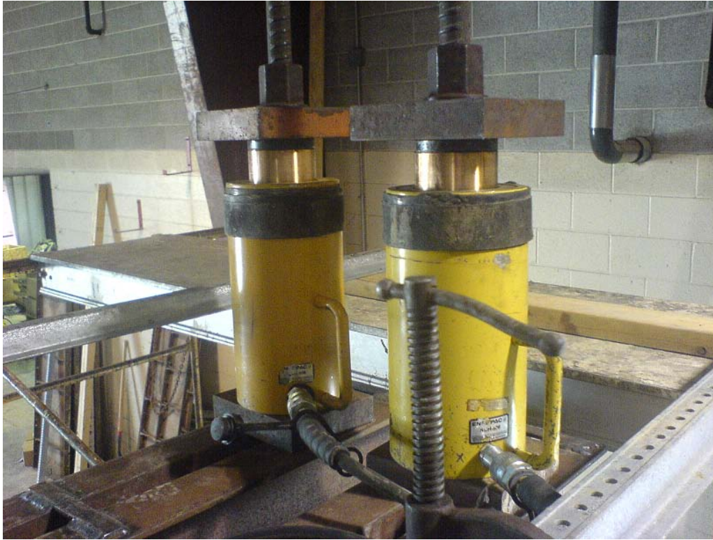
Figure 91. Photo. Hollow-core hydraulic ram bolted to the top channel beams.
