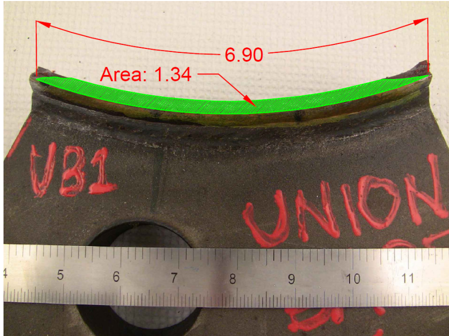
Figure 11. Photo. Specimen 1U1 fracture surface.
