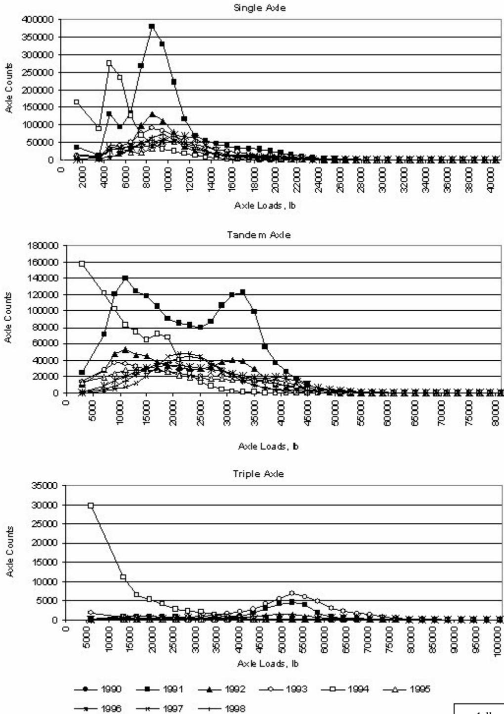
Figure 15. Use of the mean of 1991 and 1992 annual axle load spectra to obtain base annual spectrum.
