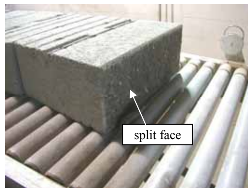
Figure 31. Photo. Split face of units.
