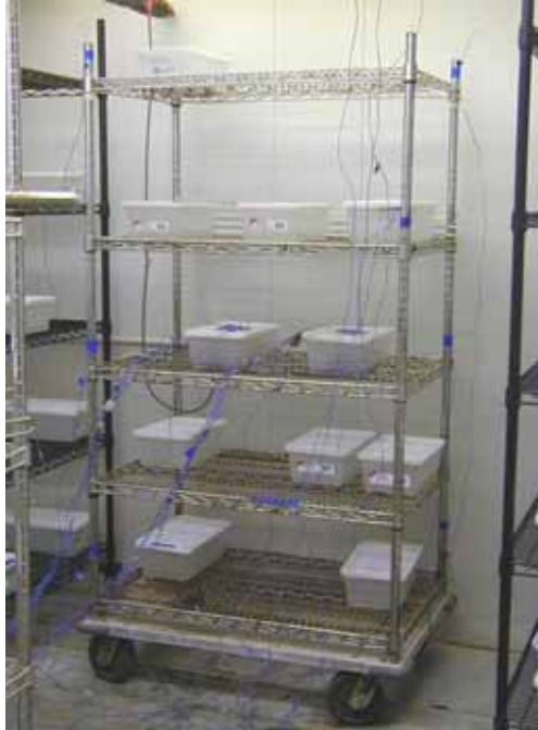
Figure 78. Photo. View of walk-in chamber with thermocouples on shelving units and suspended from ceiling.
