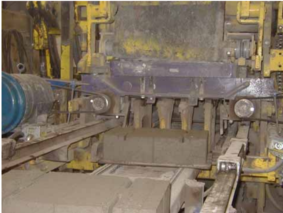
Figure 11. Photo. Demolding of SRW units during production.
