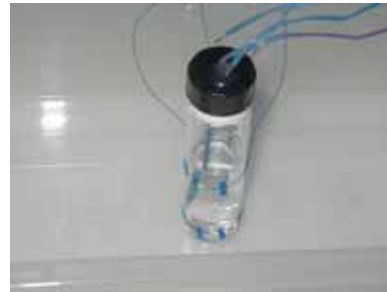
Figure 116. Photo. Water half-filled unconfined vial.
