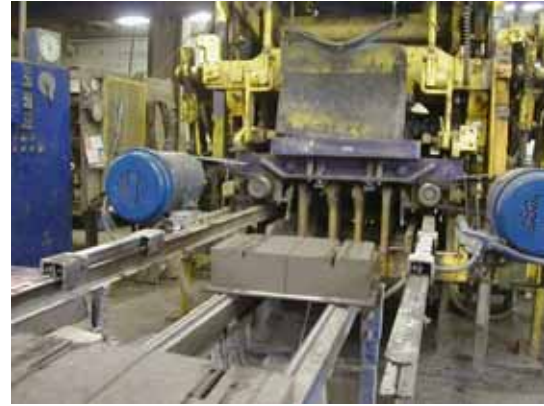
Figure 6. Photo. SRW unit immediately after compaction and demolding.
