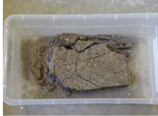
Figure 222. Photo. Comparison of water versus saline test on wall unit after 60 cycles in saline. Specimens were from a single manufacturer.
