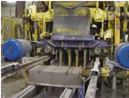
Figure 28. Photo. Units immediately after demolding.
