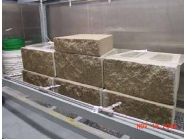
Figure 201. Photo. Typical stacking for larger SRW blocks tested in Phase II.
