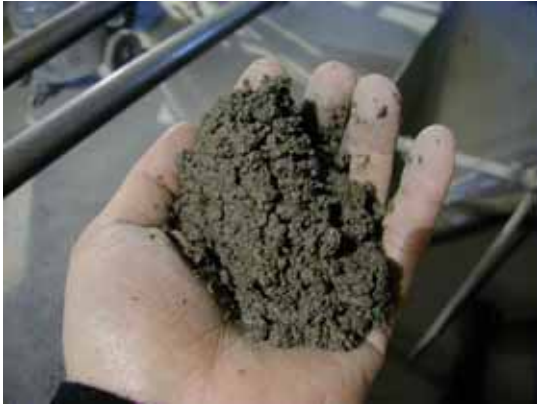
Figure 5. Photo. View of mix during production of SRW units at block plant.
