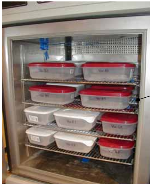
Figure 83. Photo. View of thermocouple (TC) placement with specimens in cabinet.
