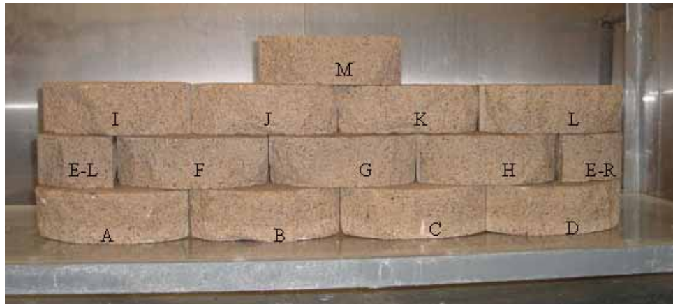
Figure 190. Photo. Freeze-thaw test setup showing SRW blocks.
