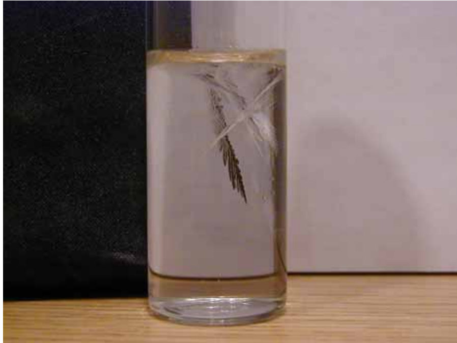
Figure 150. Photo. Half-full vial after 30 minutes of exposure in the chest freezer.
