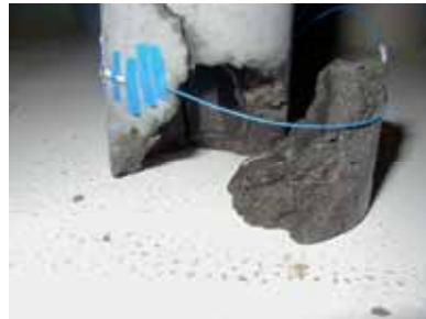
Figure 118. Photo. Water-filled, mortar-confined vial.
