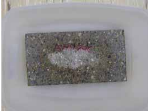
Figure 144. Photo. Specimen after 4.5-hour cold soak in walk-in freezer appears frozen solid.
