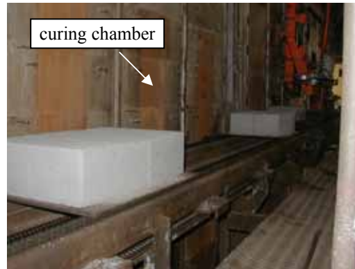
Figure 29. Photo. Units prior to entering curing chamber.
