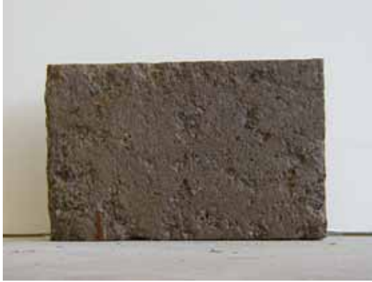
Figure 221. Photo. Comparison of water versus saline tests on wall unit after 100 cycles in water. Specimens were from a single manufacturer.
