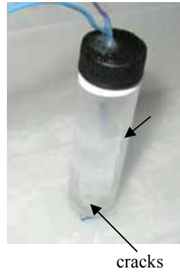
Figure 147. Photo. Half-filled vial after cooling in chest freezer.
