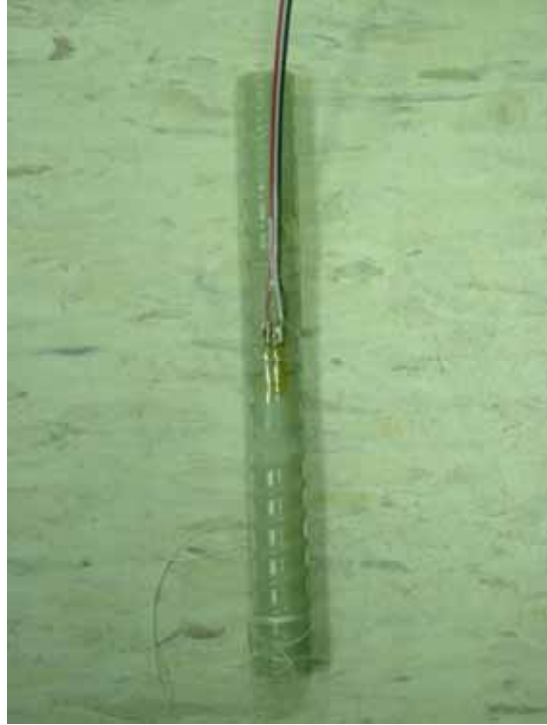
Figure 32. Photo. Number 4 GFRP rebar specimen for CTE measurement.
