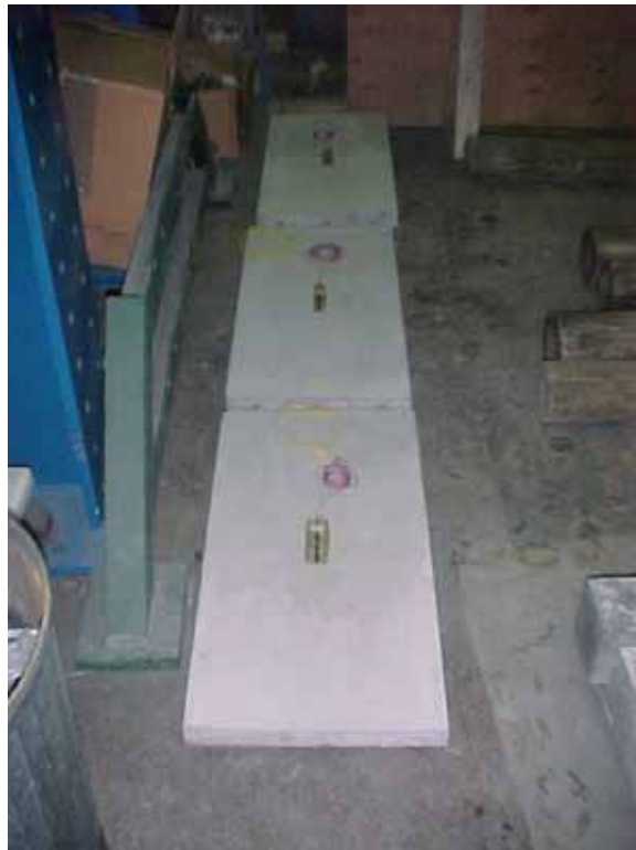
Figure 39. Photo. Concrete slabs attached with strain gages.
