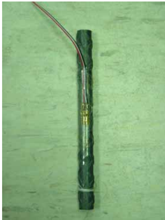
Figure 31. Photo. Number 4 steel rebar specimen for CTE measurement.
