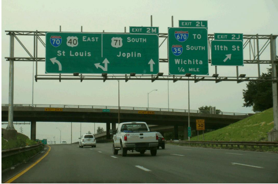
Figure 6. Photo. Truncated up-arrows on APL guide sign.
