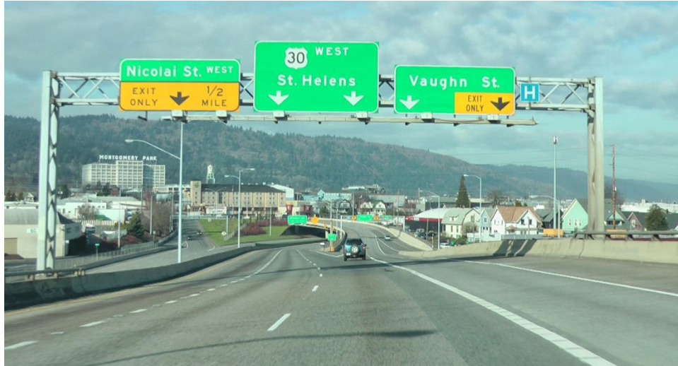
Figure 12. Photo. Example of skewed roadway perspective and difficult arrow alignment.
