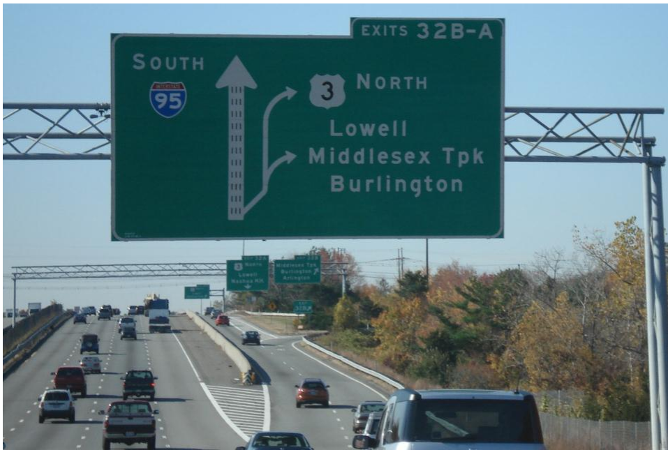
Figure 15. Photo. Example signing for a mixed system-service interchange.
