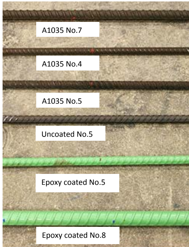
Figure 2. Photo. Reinforcing bar rib pattern.
