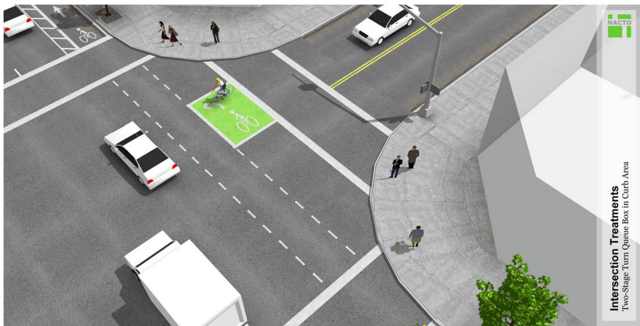
Example design of a two-stage turn queue box (NACTO Urban Bikeway Design Guide)
