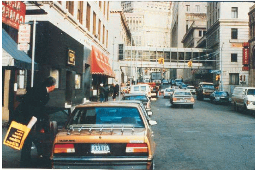
Figure 42. Grade-separated crossings can be beneficial to pedestrians under certain situations but are very costly and may not be used by pedestrians if not planned properly.
