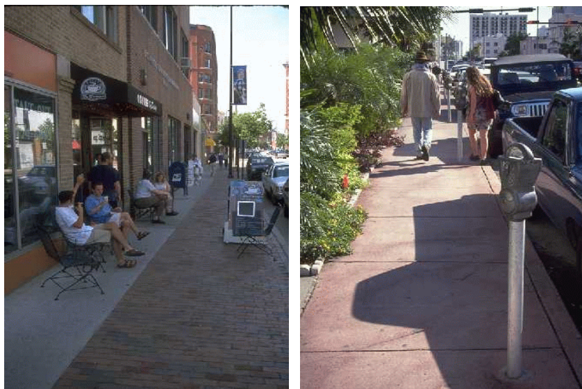
Figure 3. Pedestrian capacity of CBD sidewalks is reduced by light posts, mailboxes, parking meters, etc.
