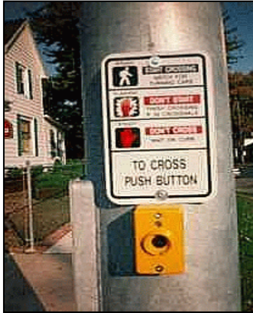
Figure 32. Illuminated pedestrian push buttons were not found to alter pedestrian crossing behavior.
