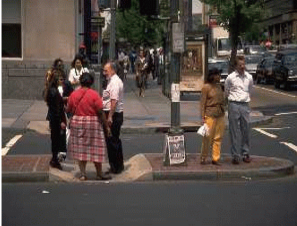
Figure 35. Raised medians and pedestrian islands may provide a measure of safety to pedestrians.
