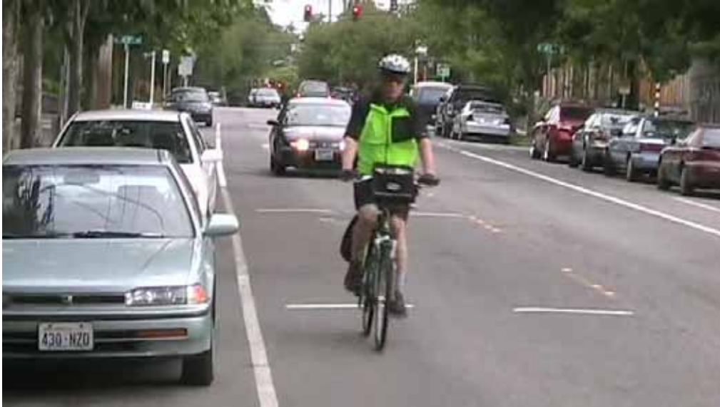
Figure 20. Photo. Typical position of bicyclist after sharrows installation.
