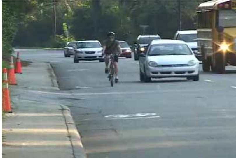
Figure 13. Photo. Motor vehicle passing a bicycle after sharrow placement with traffic in the adjacent lane.
