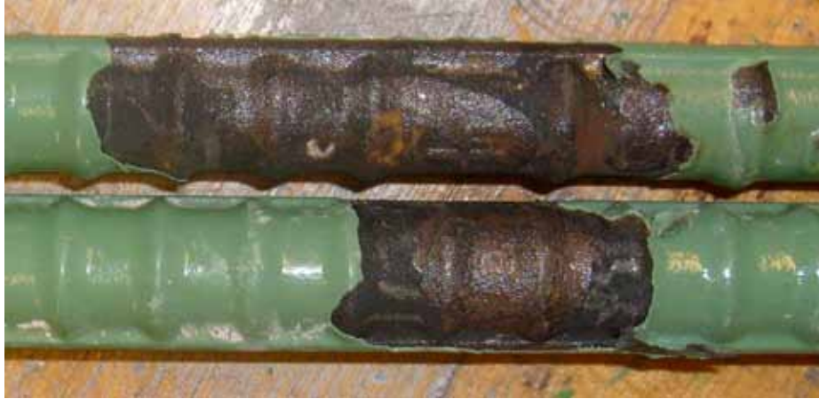
Figure 157. Photo. High adhesion DuPont™ epoxy-coated top bars from field test specimen with simulated cracks after 250 weeks.
