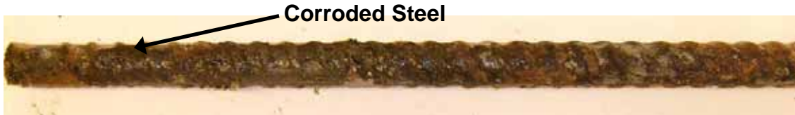
Figure 238. Photo. Bottom side of bar in specimen Zn-2, 25-mm (1-inch) cover, after autopsy.
