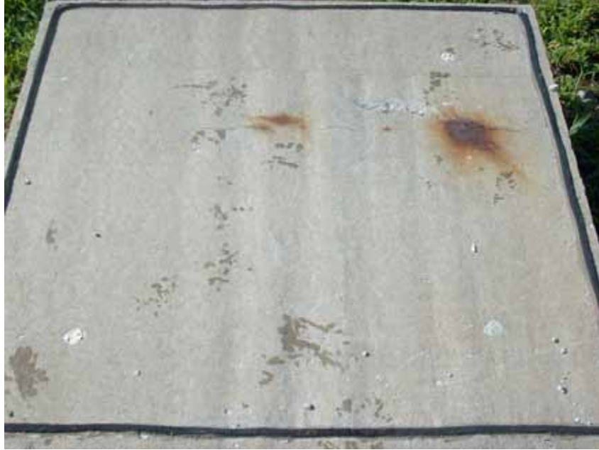
Figure 147. Photo. Field test specimen without simulated cracks containing conventional reinforcing steel at 254 weeks.
