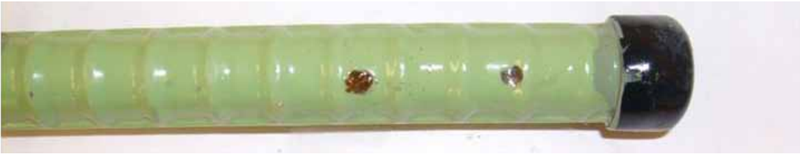
Figure 208. Photo. Rapid macrocell test, M-ECR-1, 5 weeks, before disbondment test.
