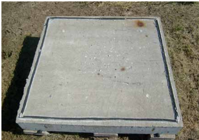
Figure 146. Photo. Field test specimen without simulated cracks containing conventional reinforcing steel at 250 weeks.
