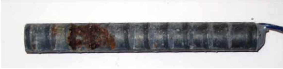
Figure 47. Photo. Conventional anode bar after removal of mortar at 15 weeks.
