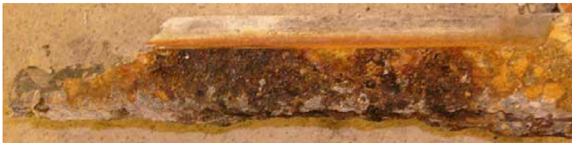
Figure 239. Photo. Side view of specimen Zn-4, 25-mm (1-inch) cover, after autopsy.
