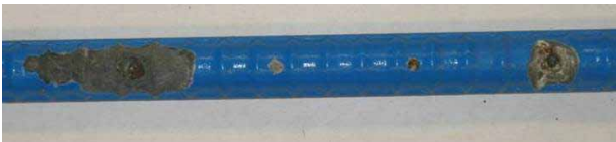
Figure 109. Photo. MC top bar with holes penetrating both epoxy and zinc from southern exposure specimen after 96 weeks.
