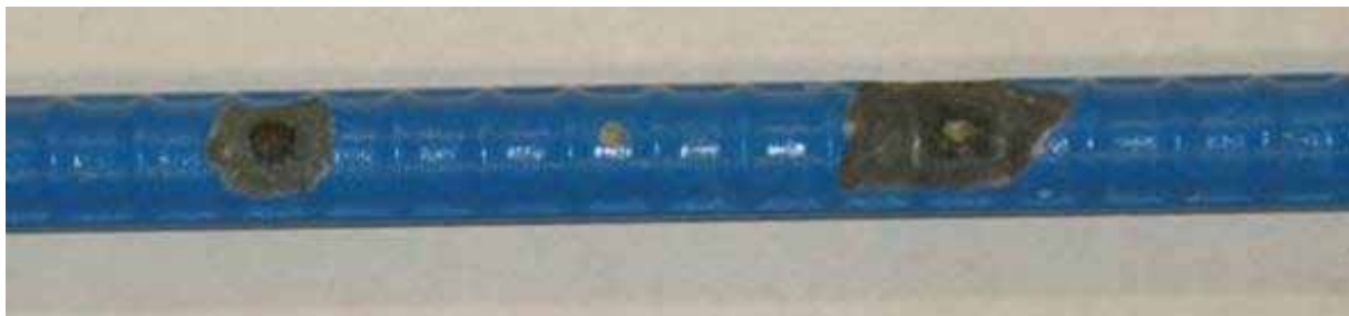
Figure 108. Photo. MC top bar with holes through epoxy only from southern exposure specimen after 96 weeks.
