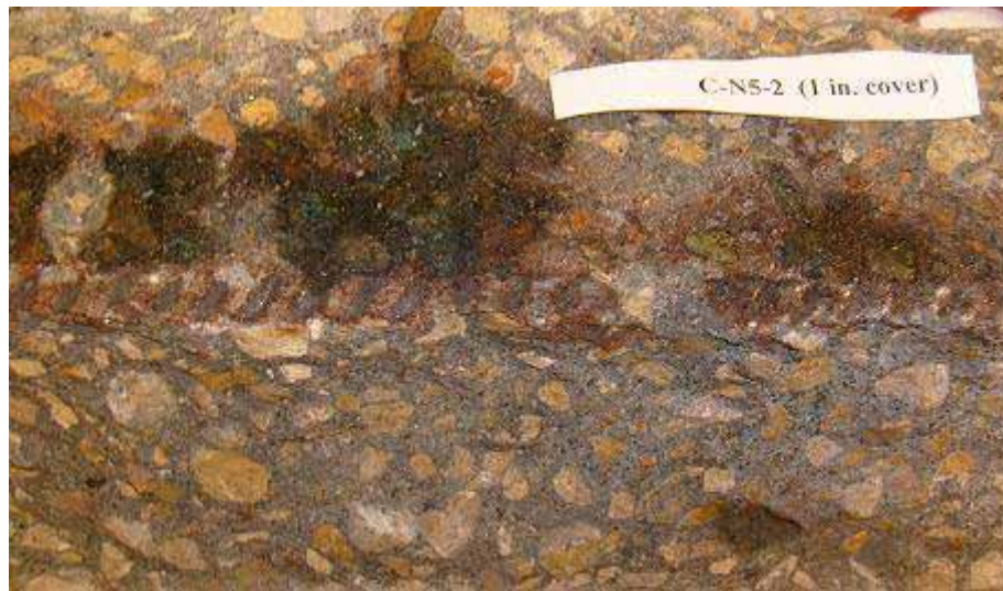
Figure 236. Photo. Top view of specimen Conv.-2, 25-mm (1-inch) cover, after autopsy.
