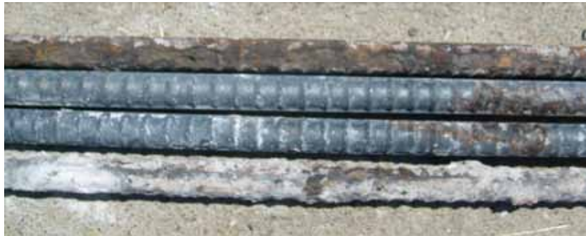
Figure 151. Photo. Top bars from field test specimen with simulated cracks containing conventional reinforcing steel at 250 weeks.
