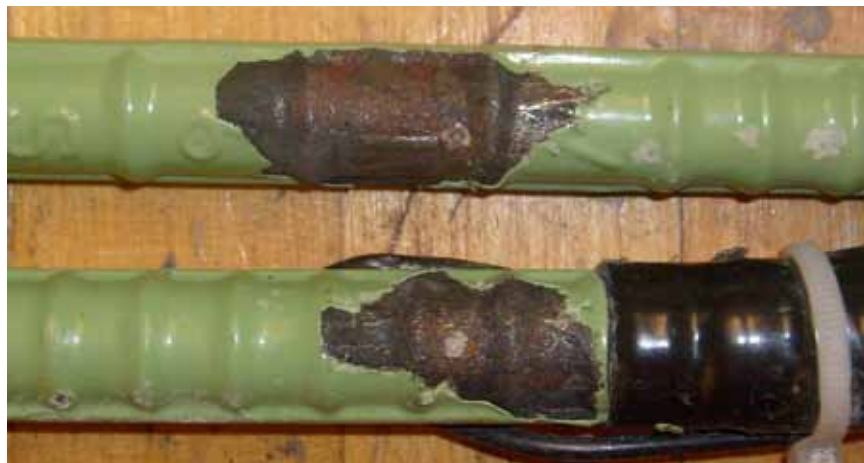
Figure 156. Photo. Conventional epoxy-coated top bars from field test specimen containing Rheocrete® 222+ corrosion inhibitor without simulated cracks after 254 weeks.
