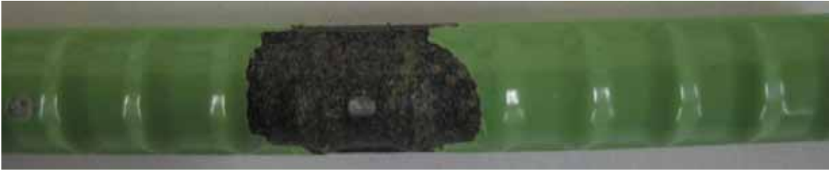
Figure 104. Photo. Conventional epoxy-coated bar from figure 103 after disbondment test.
