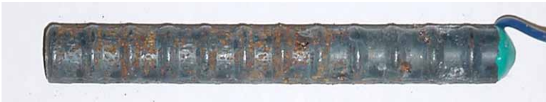
Figure 36. Photo. Bare conventional anode bar at 15 weeks showing corrosion products that formed below the surface of the solution.
