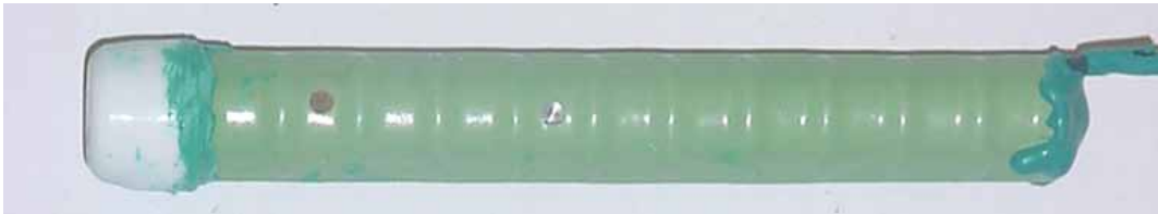
Figure 37. Photo. Bare ECR anode bar at 15 weeks showing corrosion products that formed at holes through the epoxy.
