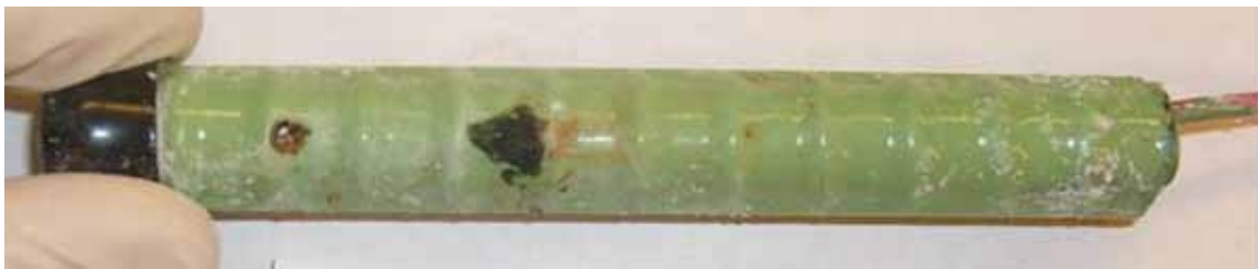
Figure 210. Photo. Rapid macrocell test, M-ECR-13, 40 weeks, before disbondment test.
