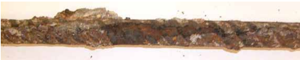
Figure 233. Photo. Top side of bar in specimen Conv.-3, 51-mm (2-inch) cover, after autopsy.
