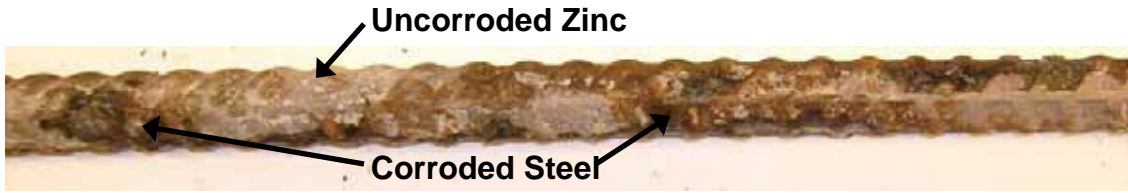
Figure 237. Photo. Top side of bar in specimen Zn-2, 25-mm (1-inch) cover, after autopsy.
