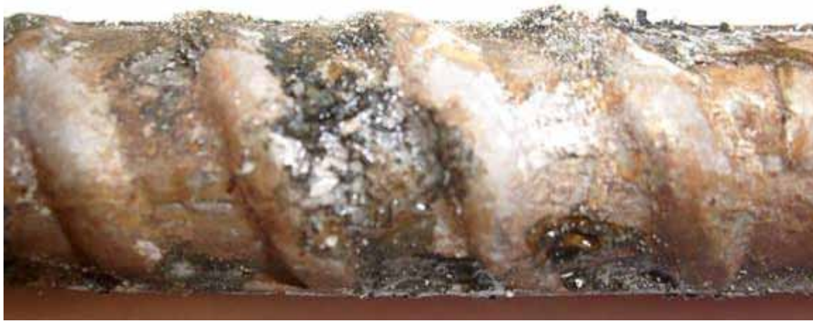
Figure 243. Photo. Detail of top side of galvanized reinforcement, 25-mm (1-inch) cover, after autopsy at crack initiation.
