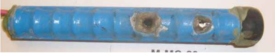
Figure 216. Photo. Rapid macrocell test, M-MC-23, 40 weeks, after disbondment test.
