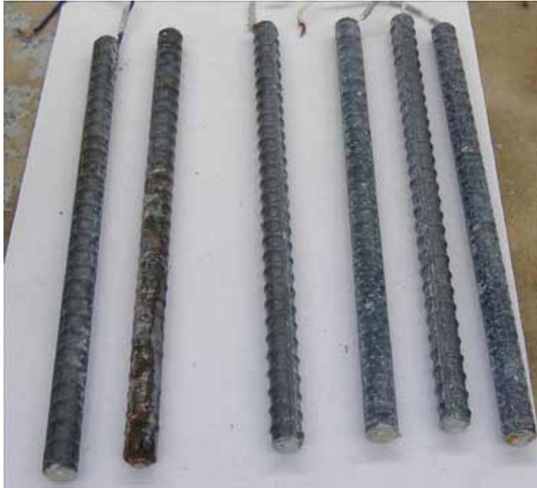
Figure 101. Photo. Conventional steel bars from southern exposure specimen after 96 weeks.
