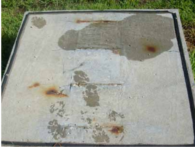
Figure 149. Photo. Field test specimen with simulated cracks containing conventional reinforcing steel at 254 weeks.
