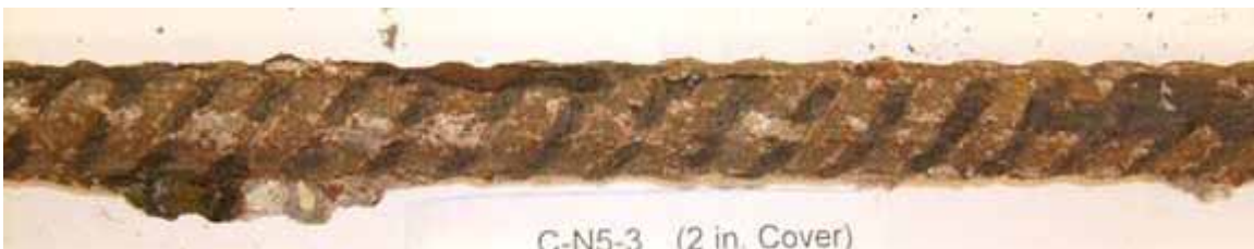
Figure 234. Photo. Bottom side of bar in specimen Conv.-3, 51-mm (2-inch) cover, after autopsy.
