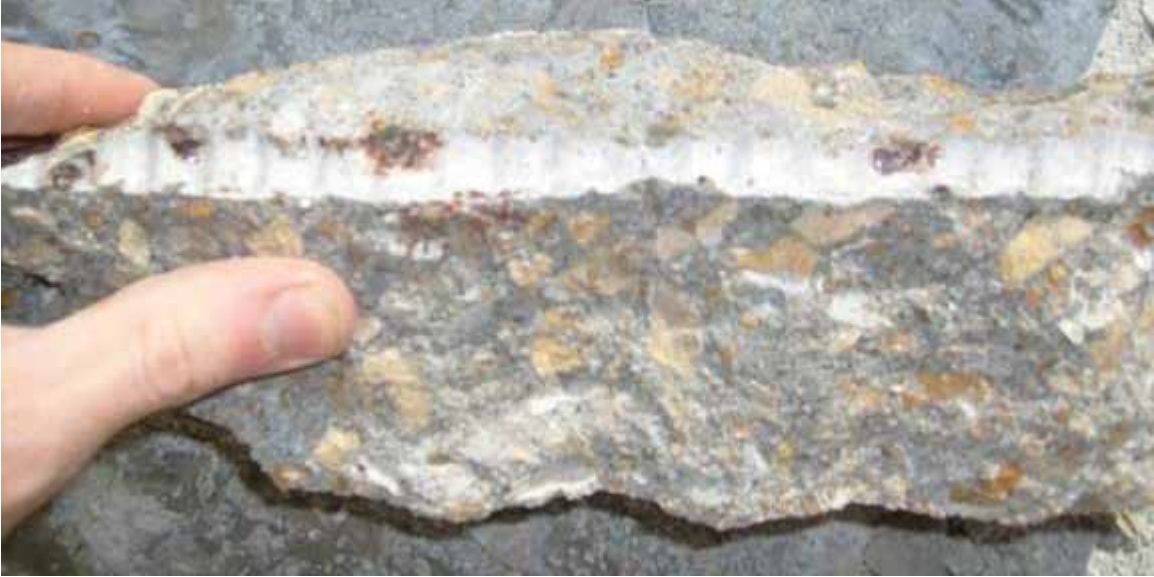
Figure 248. Photo. Concrete surrounding test bar from specimen ECR-2h-V-1.
