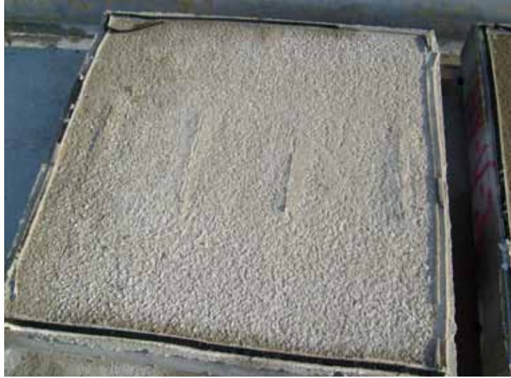
Figure 155. Photo. Field test specimen with simulated cracks containing conventional ECR and Hycrete™ corrosion inhibitor at 254 weeks.
