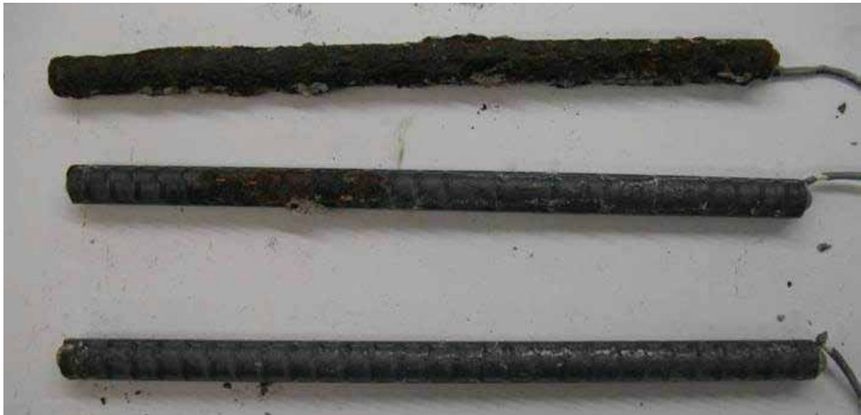
Figure 102. Photo. Conventional steel bars from cracked beam specimens after 96 weeks.
