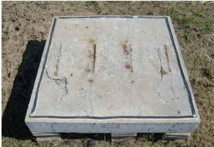
Figure 148. Photo. Field test specimen with simulated cracks containing conventional reinforcing steel at 250 weeks.
