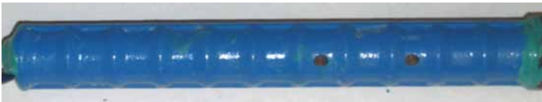
Figure 38. Photo. Bare MC anode bar with only epoxy penetrated at 15 weeks showing corrosion products that formed at holes through the epoxy.
