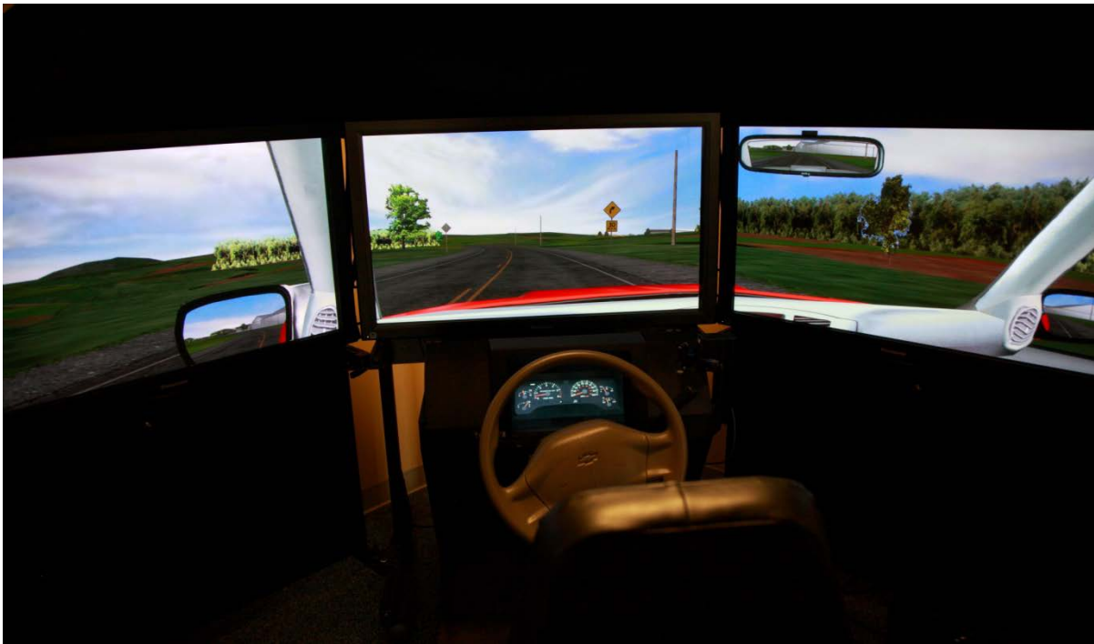
Figure 4. Photo. Driving simulator with three 42-inch plasma displays and driving buck.
