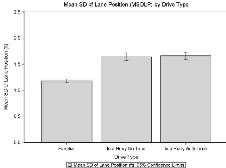
Figure 18. Graph. MSDLP by drive type for combined curve degree, in a hurry.
