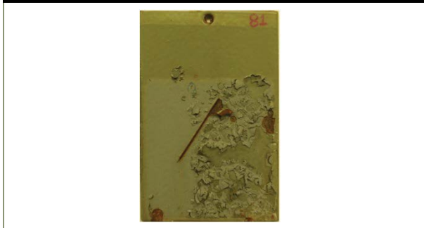
Figure 4. ZnE/LE coating system after 3,600 h in ALT.
