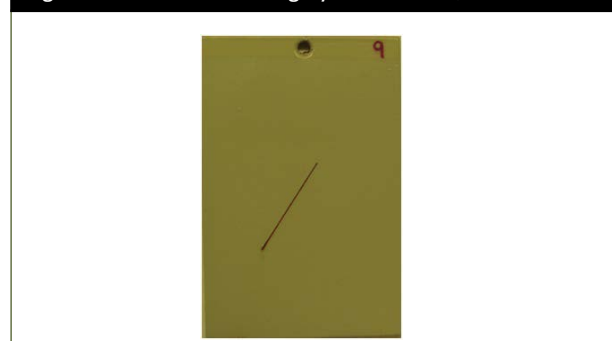
Figure 3. IOZ/E/PU coating system after 3,600 h in ALT.
