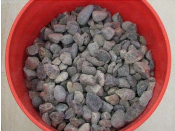
Figure 8. Photo. Las Placitas gravel aggregate as received
