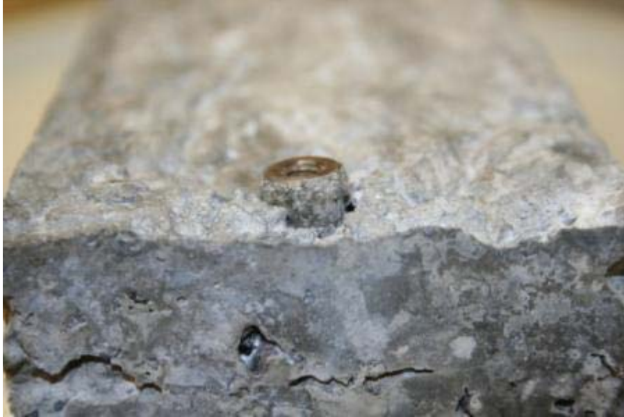
Figure 40. Photo. Cast accelerometer attachment for Sample 2
