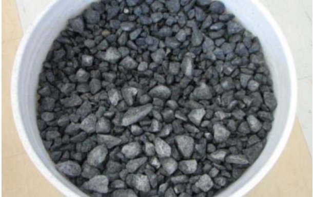
Figure 10. Photo. Adairsville limestone (coarse) aggregate as received
