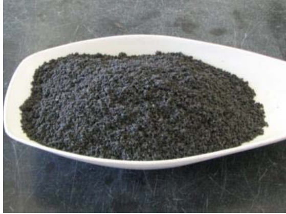
Figure 11. Photo. Adairsville limestone (fine) aggregate as received
