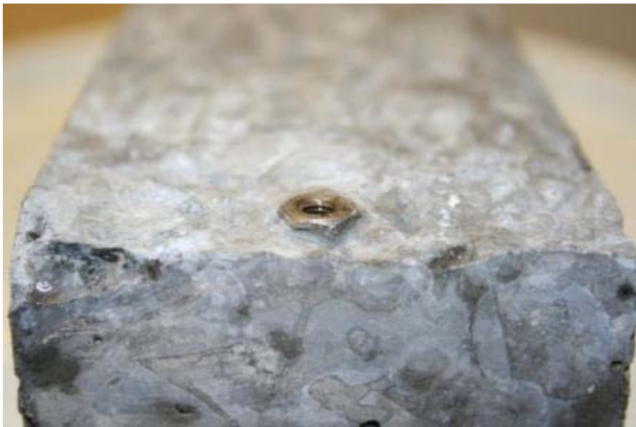
Figure 41. Photo. Cast accelerometer attachment for Sample 3
