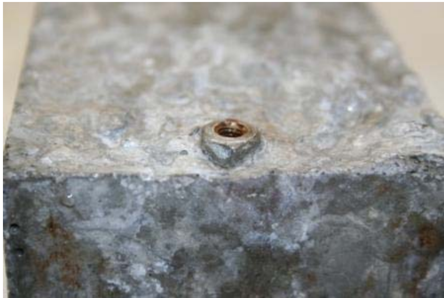
Figure 39. Photo. Cast accelerometer attachment for Sample 1
