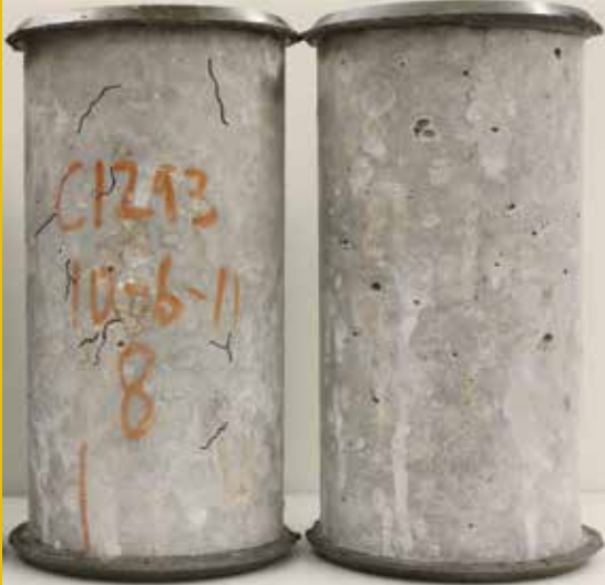
Two concrete samples using equivalently reactive aggregate. Left, ASR-damaged concrete with cracks marked; right, crack-resistant HyFRC for concrete strength and stiffness retention.
