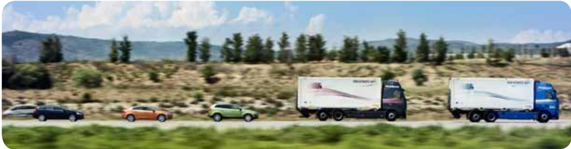
Figure 2. Photo. SARTRE demonstration of three automated cars and one automated truck following the lead truck in a platoon (May 2012).
