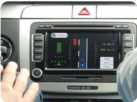
Figure 10. Photo. Volkswagen's Temporary Auto Pilot display, showing three levels of automation choices in lower right corner.
