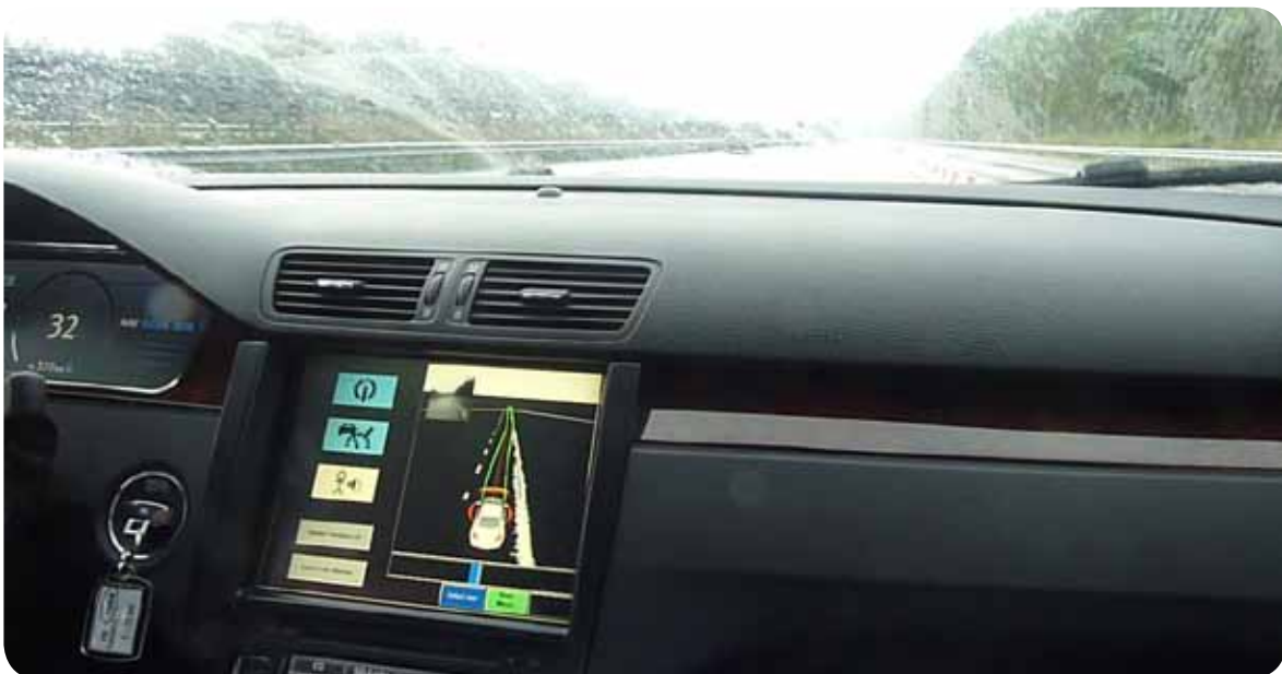
Figure 15. Photo. Roadworks Assistant driver-vehicle interface, showing three levels of automation on left side of screen.
