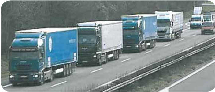
Figure 32. Photo. Four-truck KONVOI platoon driving at 10-m (33-ft) gaps between trucks on a German autobahn.
