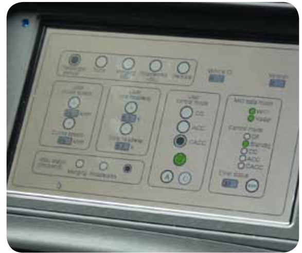
Figure 26. Photo. Touch-screen control panel for adjusting parameters of a cooperative adaptive cruise control (CACC) test vehicle. NOTE: RSU = roadside units, CC = cruise control, ACC = adaptive cruise control.
