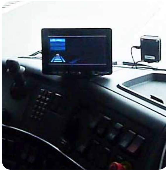
Figure 12. Photo. Automated Queue Assistance (AQuA) driver interface for heavy trucks.
