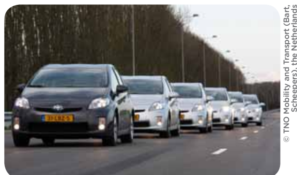
Figure 25. Photo. Cooperative adaptive cruise control platoon of Toyota Prius vehicles developed as part of the Connect and Drive Project.
