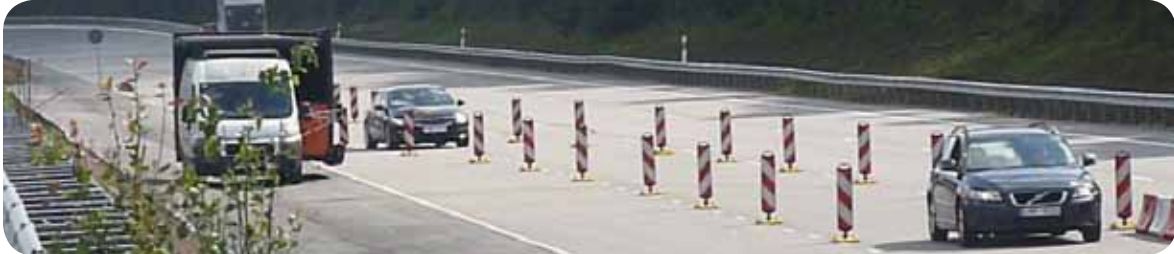
Figure 14. Photo. An Automated Roadworks Assistant vehicle follows a lead vehicle between pylons and maintains separation from a truck.
