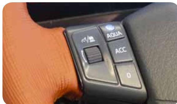
Figure 11. Photo. Steering wheel controls for Volvo Automated Queue Assistance (AQuA) for heavy trucks.
