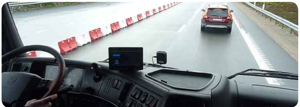
Figure 13. Photo. Automated Queue Assistance (AQuA) system demonstration for low-speed automation in a truck.
