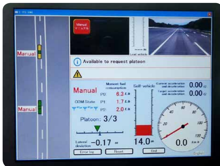
Figure 41. Photo. In-vehicle display screen of a following truck in the Energy ITS platoon.
