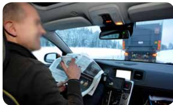
Figure 3. Photo. Reading a newspaper while being driven automatically in the platoon behind the lead truck (December 2010).
