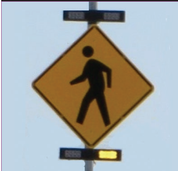
Figure 2. RRFB bar locations tested. (Note that only one bar unit was activated at a time.)
