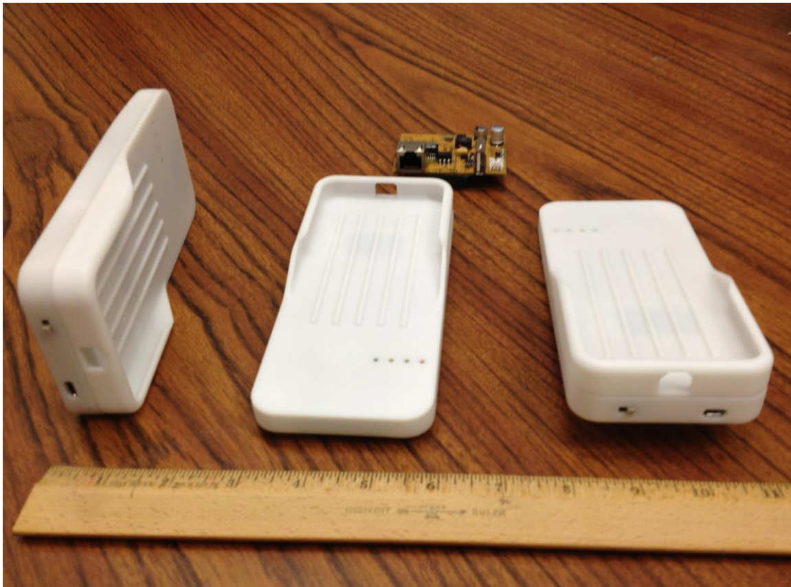
Figure 7-7. Nomadic Device DSRC Radio Module
