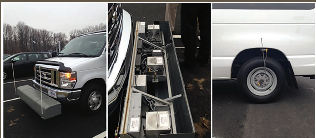
Figure 9. Inertial profilometer vehicle (left), sensor bar with cover open (center), and distance measurement instrument (right).
