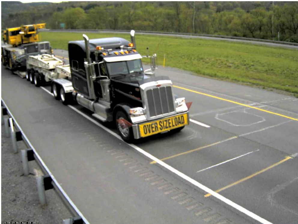
Figure 30. Photo. Eleven-axle Class 13 truck at Pennsylvania site.
