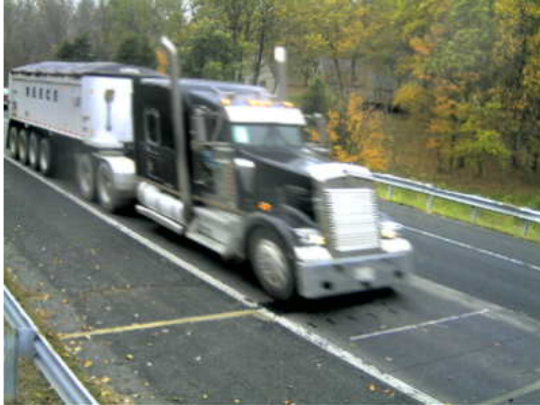
Figure 33. Photo. Seven-axle Class 10 truck at Maryland site.
