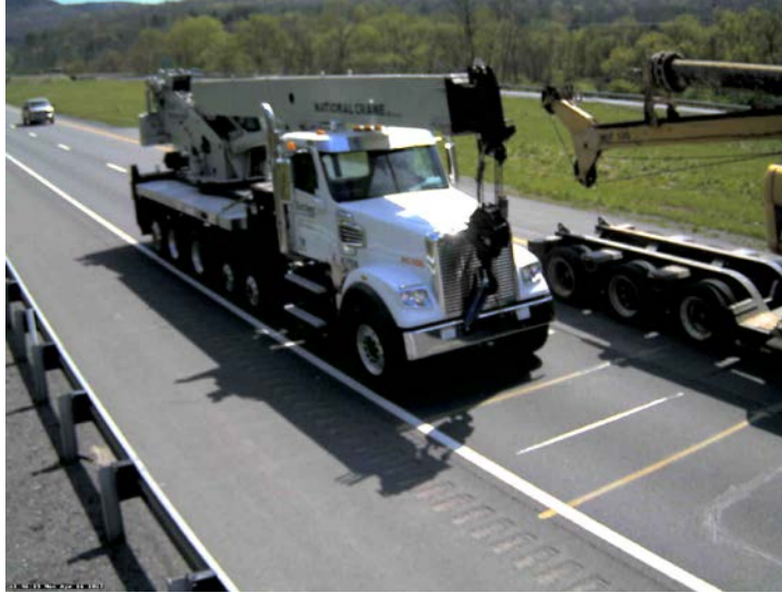
Figure 27. Photo. Six-axle Class 7 truck at Pennsylvania site.
