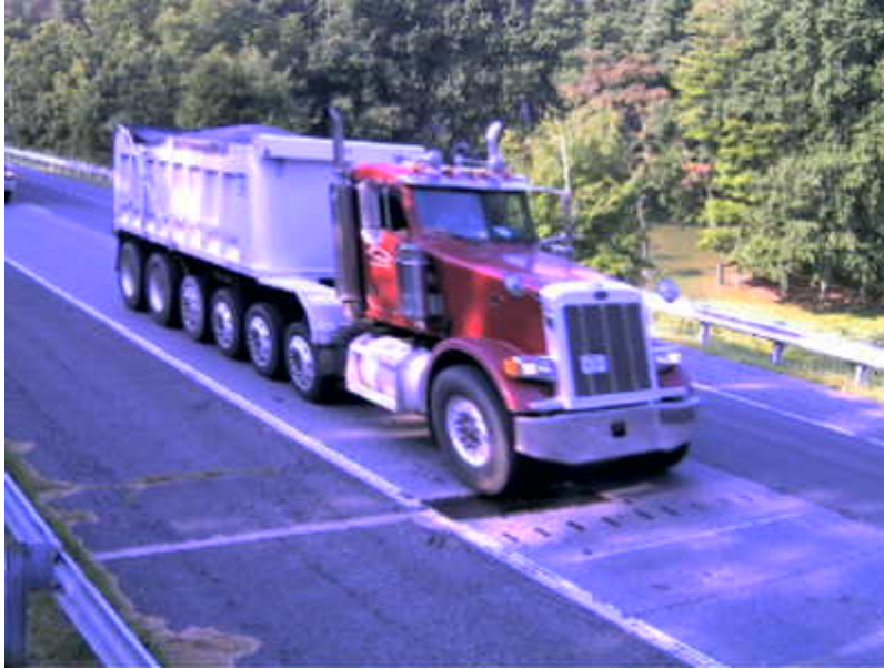
Figure 31. Photo. Seven-axle Class 7 truck at the Maryland site.
