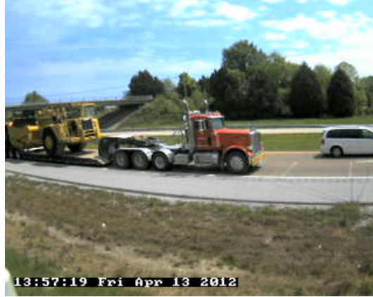
Figure 36. Photo. Class 10 truck, no second articulated connection.
