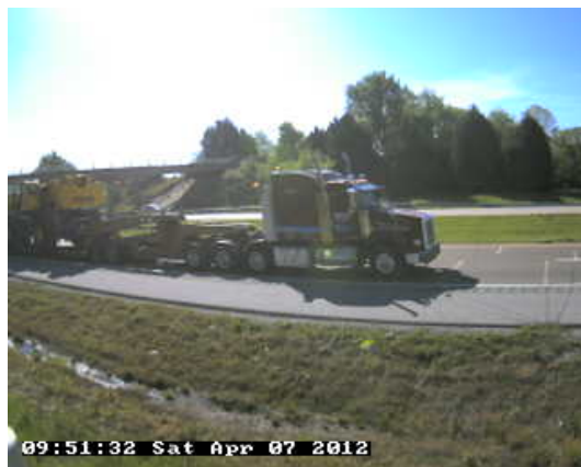
Figure 37. Photo. Class 13 truck with a second articulated connection.
