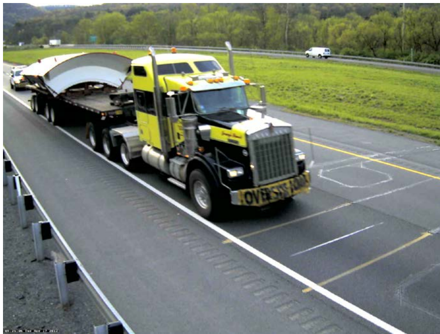
Figure 29. Photo. Image 2 of eight-axle Class 10 truck at Pennsylvania site.
