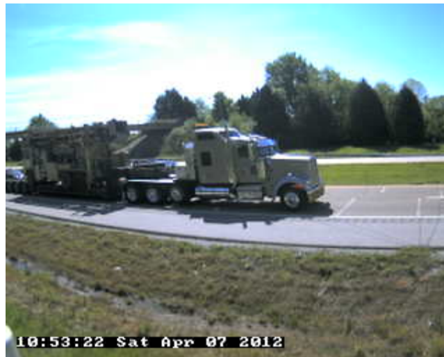
Figure 34. Photo. Seven-axle Class 10 truck in Tennessee.
