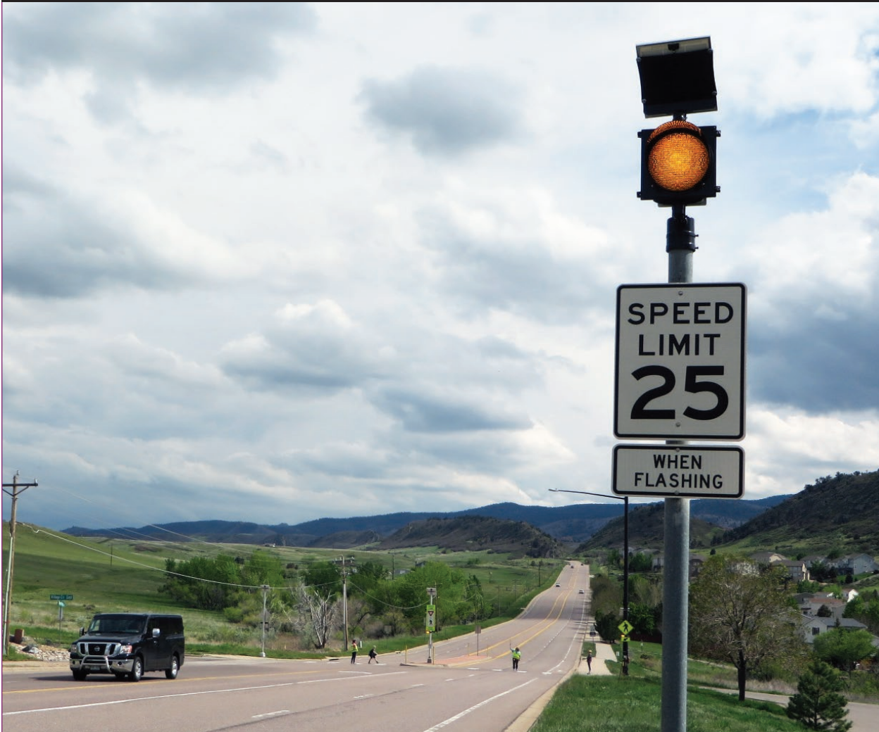
Figure 3. Example of speed limit sign assembly used at three sites in Colorado.
