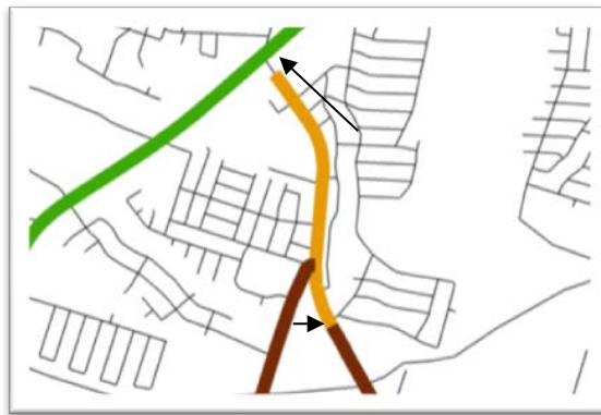
Figure 4-2: Example of Shifting due to Inconsistency between Tabular Event Data and Geospatial Data
