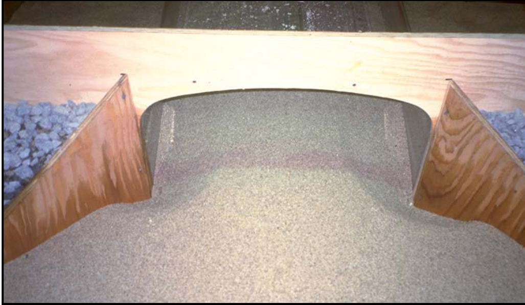
Figure 6.17. Arched model with wing walls (FHWA 2003a).
