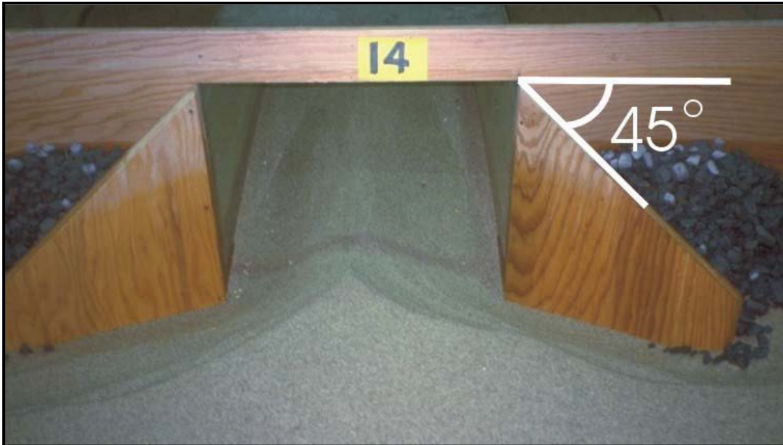
Figure 6.16. Rectangular model with wing walls (FHWA 2003a).
