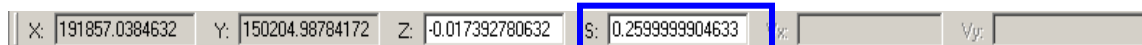
Figure B 6.4-3. Toolbar at top of SMS window giving the X,Y,Z, and S (scalar) value of each cell or an average of the cells selected.
