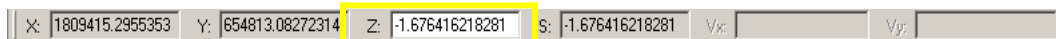
Figure 6. Toolbar at top of SMS window containing the X, Y, Z, and S (scalar quantity) of the selected cell or an average Z of multiple selected cells.
