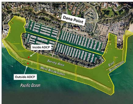
Figure 1 Bathymetric and LiDAR survey area. Red dots show the location of two ADCPs.
