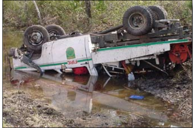
A brush truck driven by Firefighter Edward Orlando Peters rolled over into a water-filled ditch as a result of a tire blowout.
