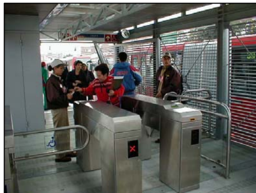
FIGURE 3.23 – Station Access and Off-board Fare Payment
