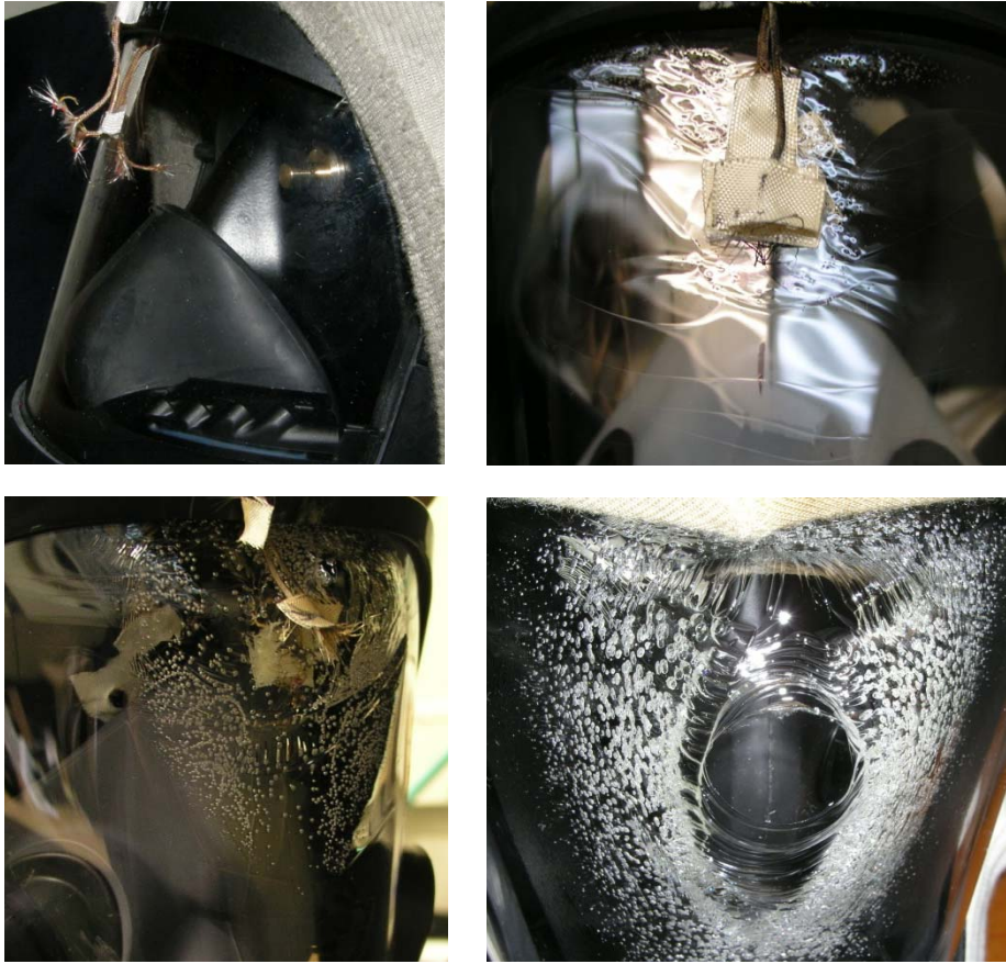
Figure 1 – Photos of example facepiece lenses; pre-exposure with the thermocouples placed on the lens (top left), post-exposure with cracks/crazing (top right), post-exposure with bubbling (bottom left), and post-exposure with deformation causing a hole and bubbling (bottom right).
