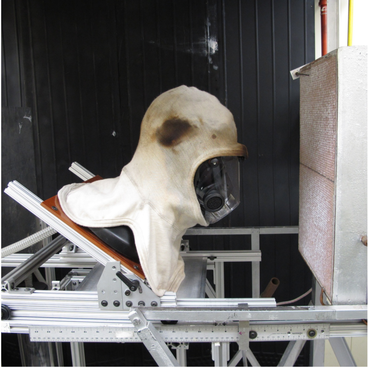
Figure 21. Headform and facepiece mounted on cart and positioned in front of radiant panel. Facepiece lens is parallel with radiant panel, and located approximately 178 mm (7.0 in) from panel surface.
