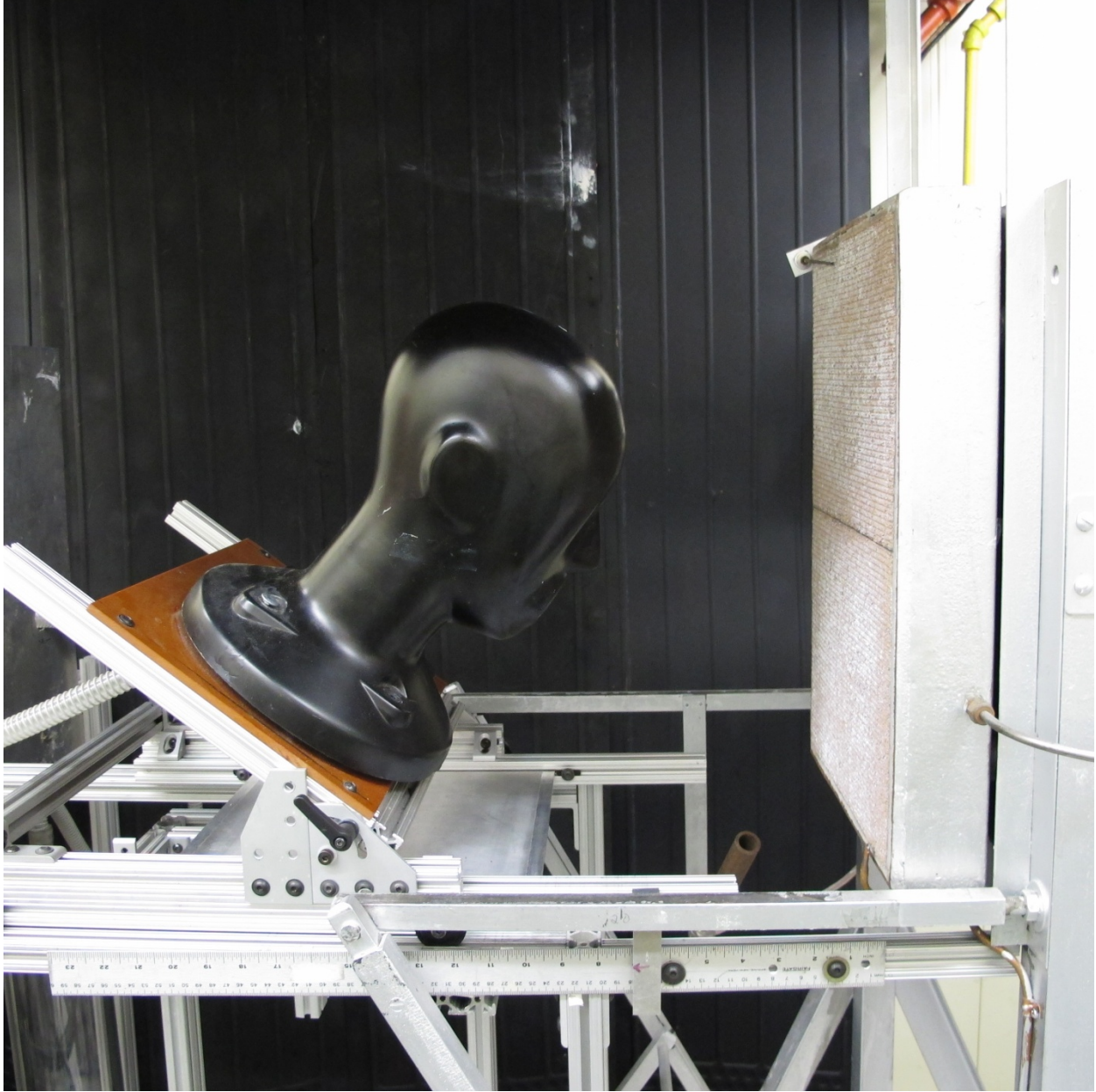
Figure 20. Headform mounted on cart and positioned in front of radiant panel.
