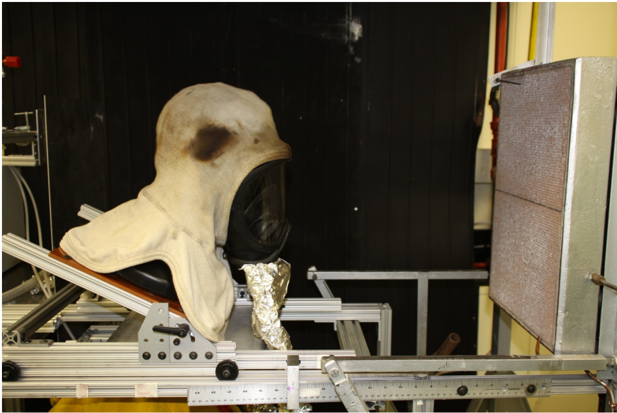
Figure 2. Radiant panel apparatus with SCBA facepiece and hood installed on adjustable headform frame.
