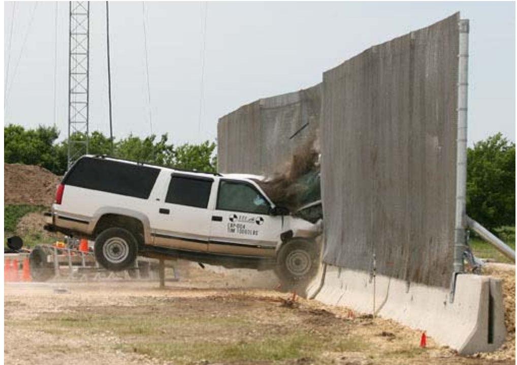
Figure 4: Fence Crash Test at Fence Lab
