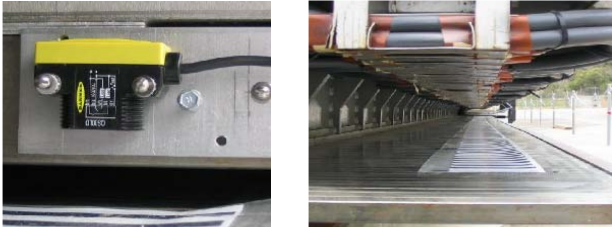
Figure 7. Laser sensor (left) and optical tape (right)
