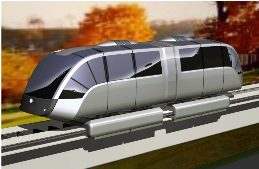
Figure 1-1 General Atomics Urban Maglev vehicle uses permanent magnets arranged in a Halbach array configuration for levitation and propulsion
