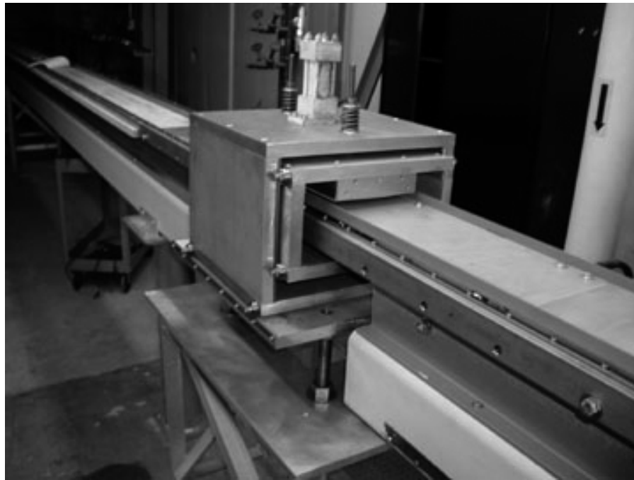
Figure 3.4-2 Photograph of test rig, showing assembly within which Halbach arrays are mounted, vertical force sensor, and movable carrier for the laminated track
