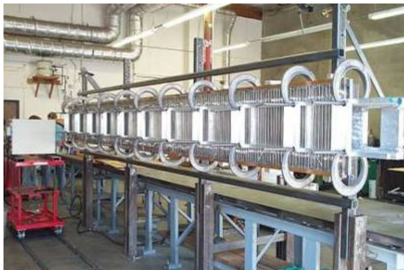
Figure 1-7 Semi-automated soldering process for the litz track enables consistent joint resistance
